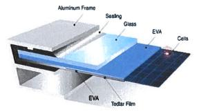
Figure 2: Components of crystalline silicon panels.
