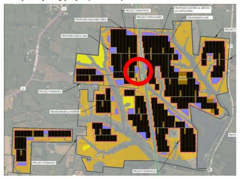
It is depicted on the revised site plan below as the small orange line between the project substation and the utility switchyard.
