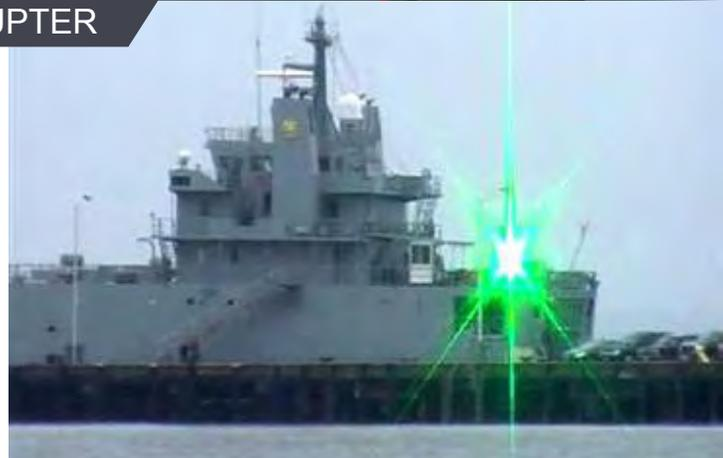
*U.S. Navy maritime expeditionary security group uses a laser distracter to warn a simulated vessel to keep its distance.*
