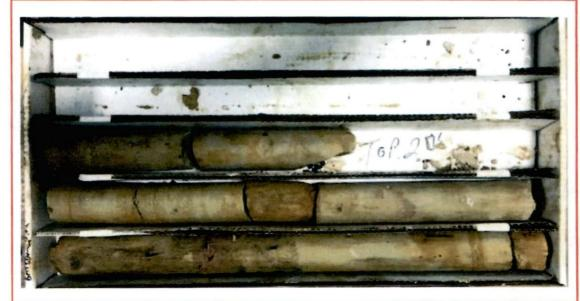
PHOTO #2 – Rock core sample at B-1 from about 20 to 25 feet below existing grade (bottom of the core at lower left corner)
