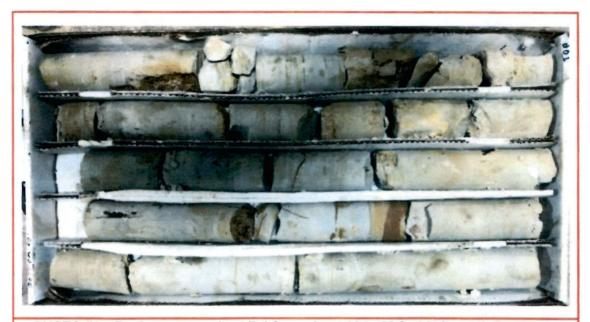
PHOTO #1 – Rock core sample at B-1 from about 10 to 20 feet below existing grade (top of the core at upper right corner)
