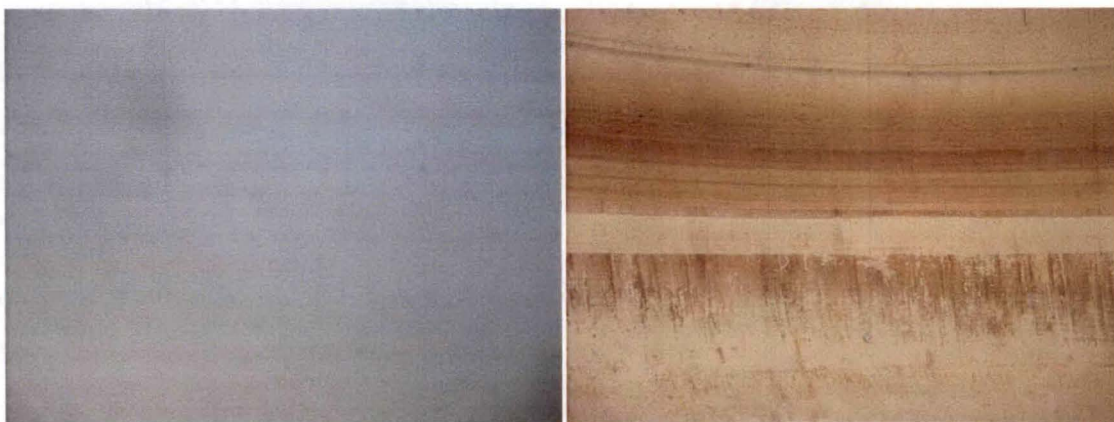
Figure 1: A chemically cleaned tank (left) compared to a pressure washed tank (right).
