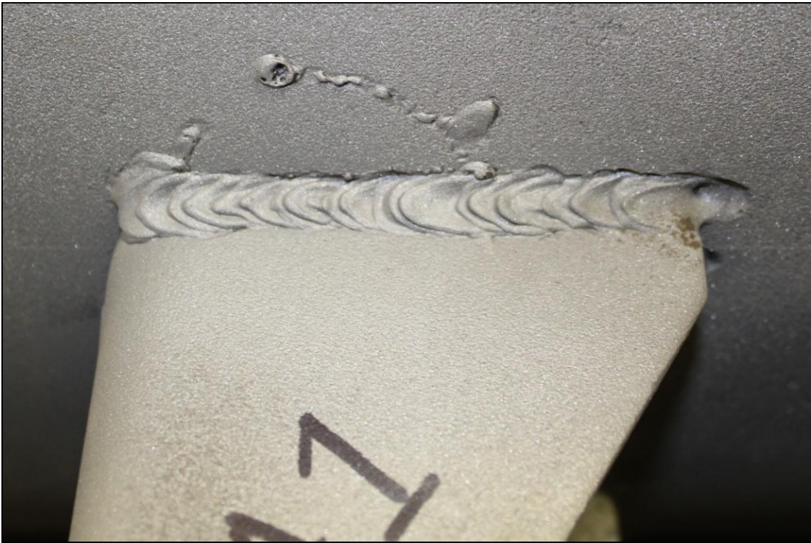
Figure 5. Image of the Lug A1 exterior top weld which exhibited substantial fusion except for some undercut and arc strikes.
