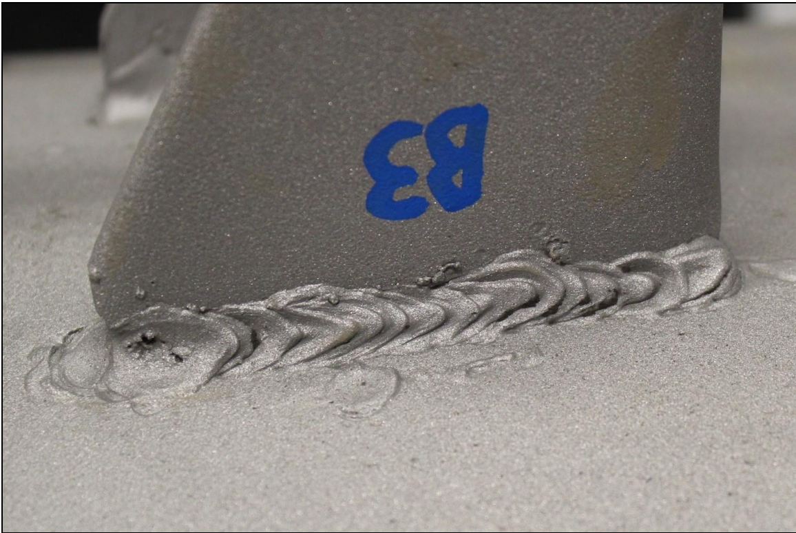
Figure 11. Image of the Lug B3 exterior bottom weld which exhibited substantial fusion except for arc strikes, porosity, and spatter.
