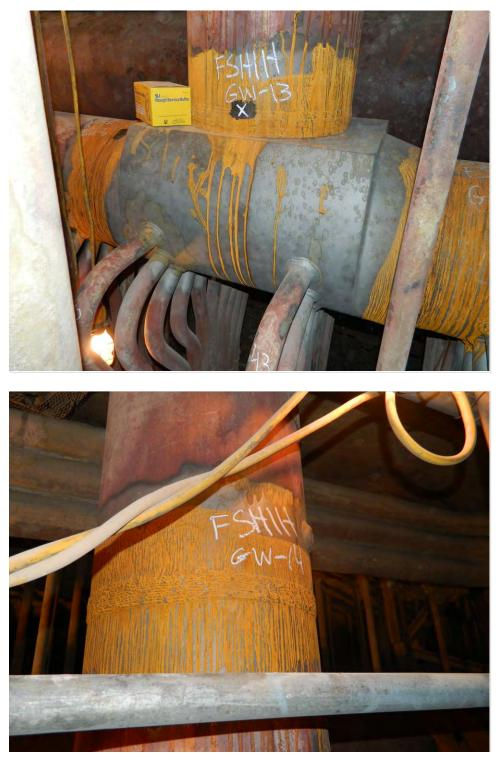
Fig. 39. Photographs of girth weld Nos. GW-13 and GW-14 on the Finishing Superheater Inlet header
