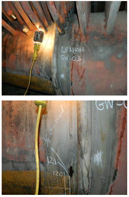
Fig. 90. Photographs of the indications on girth weld No. GW-3 of the LP Reheat Outlet header.
