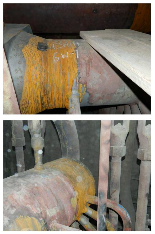
Fig. 36. Photographs of girth weld Nos. GW-7 and GW-8 on the Finishing Superheater Inlet header.
