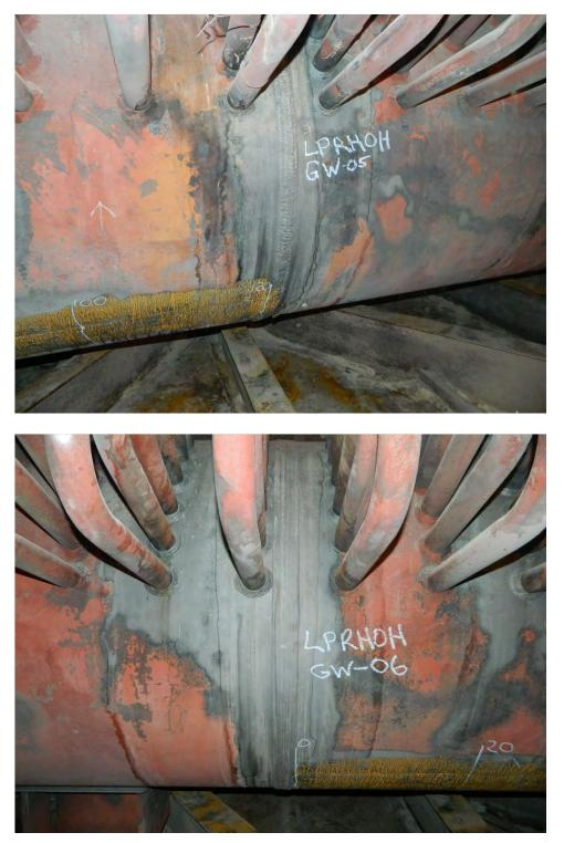
Fig. 86. Photographs of girth weld Nos. GW-5 and GW-6 on the LP Reheat Outlet header
