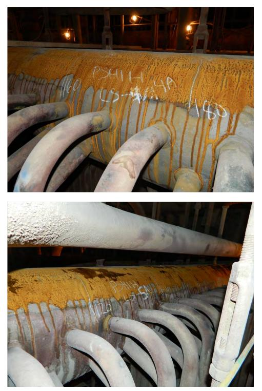
Fig. 4. Photographs of seam weld Nos. LS-4A and LS-5A on the Platen Superheater Inlet header.
