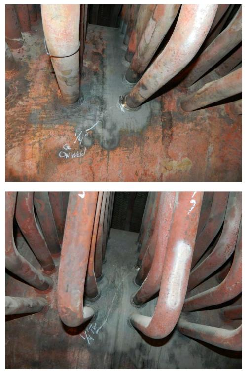
Fig. 91. Photographs of the indications on the tube stubs of the LP Reheat Outlet header.
