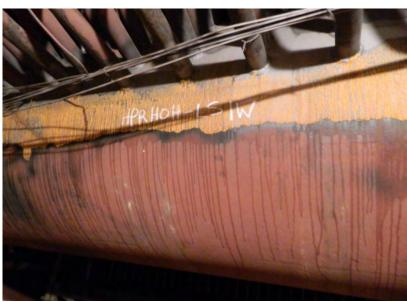
Photographs of seam weld Nos. LS-1W, LS-2W, and LS-2E on the HP Reheat Outlet header.
