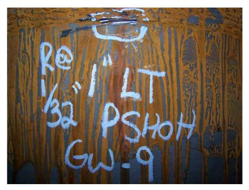
Fig. 18. Photograph of indication removal on girth weld No. GW-9 on the Platen Superheater Outlet header.
