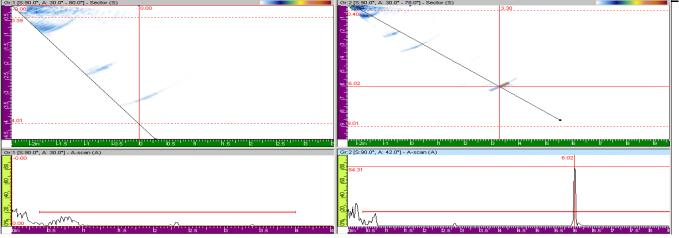
Image of typical 360° non-relevant root signal/root geometry. Limited scanning accessibility due to tube stubs. No relevant indications detected.
