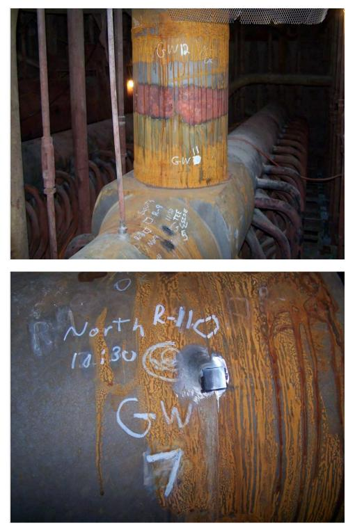
Fig. 17. Photographs of the inspection locations on the Platen Superheater Outlet header.
