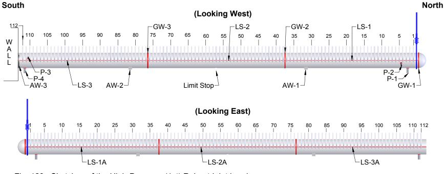
Fig. 123. Sketches of the High-Pressure (1st) Reheat Inlet header
