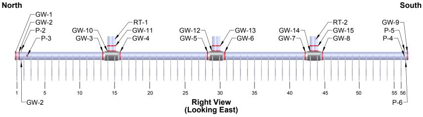
Fig. 30. Sketch of the Finishing Superheater Inlet header
