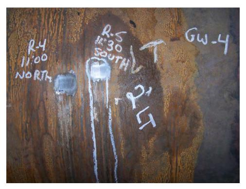
Fig. 56. Photographs of the indications in girth weld No. GW-4 on the Lower Finishing Superheater Outlet header.
