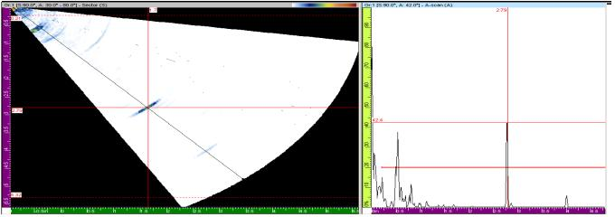
Image of typical 360° non-relevant root signal/root geometry. No relevant indications detected.
