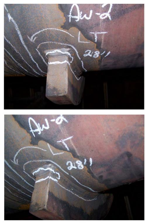
Fig. 95. Photographs of indications in attachment weld No. AW-2 on the High-Pressure Reheat Outlet header.
