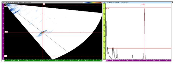
Image of typical 360° non-relevant root signal/root geometry. No relevant indications detected.
