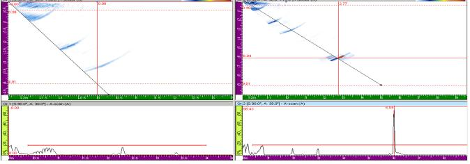
Image of typical 360° non-relevant root signal/root geometry.
