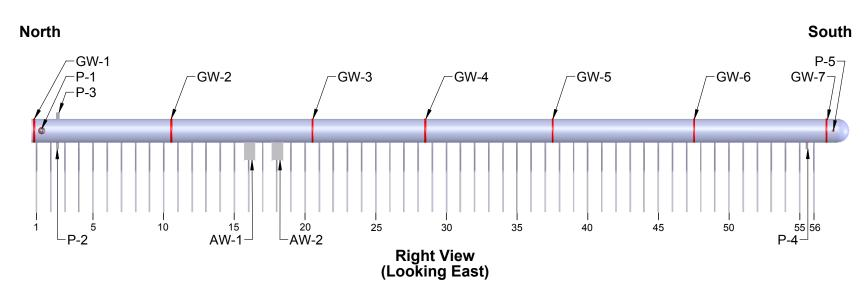
Fig. 46. Sketches of the Upper Finishing Superheater Outlet header
