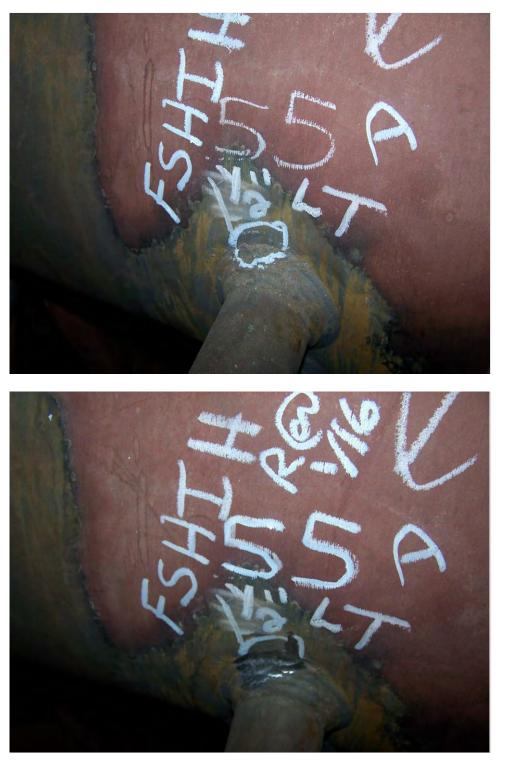
Fig. 34. Photograph of indication before and after removal in tube stub 55A on the Finishing Superheater Inlet header.
