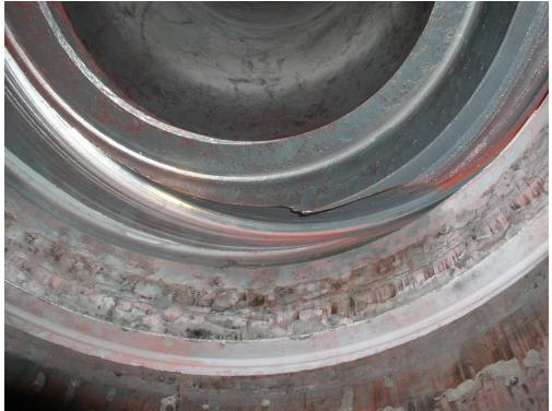
Upper Inlet Bore Damage
