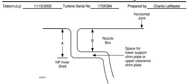
**NOTES:** On upper half box, the B dimension is to be taken with the upper clearance shim plate (or crush pins) removed. Data in inches.
