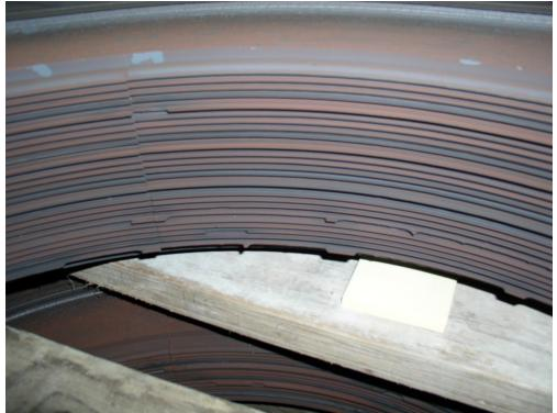
As Found Packing Damage - 2nd Stage
