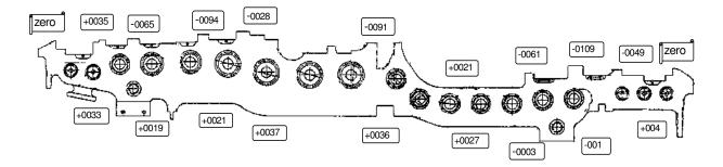
Readings taken at AEP CMS Charleston W.Va. 09-27-05 by Vince Kollin & Craig Schmotzer Inner Shell Horizontal Joint LHSheet1 AEP Mitchell Unit # 2 HP Inner Shell Upper Half Horizontal Joint Flatness Check W/ Hamar Laser
