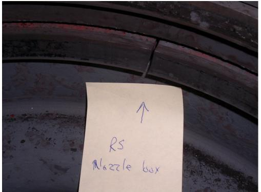
Broken Nozzle Seal Ring
