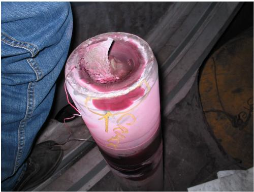
Stellite Crack Before Grinding
