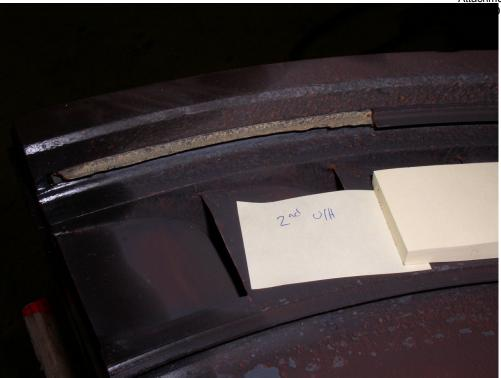
Deteriorated 2nd Stage Spill Strip
