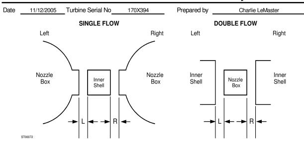
NOTE: Permanent sizes are to give proper alignment and provide specified drawing clearance.
