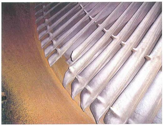
As Found Damage- Broken Blade #91
