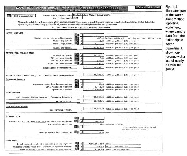
read from left-to-right, follows the path of the water supply from delivery to customer consumption (Figure 2).
