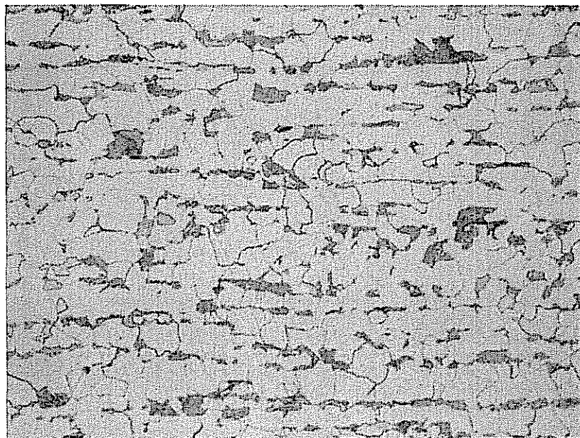
Figure 3. Typical pearlite and ferrite mid-wall microstructure at hot side of Tube W-6A, and common in all West wall tubes. 400x.
