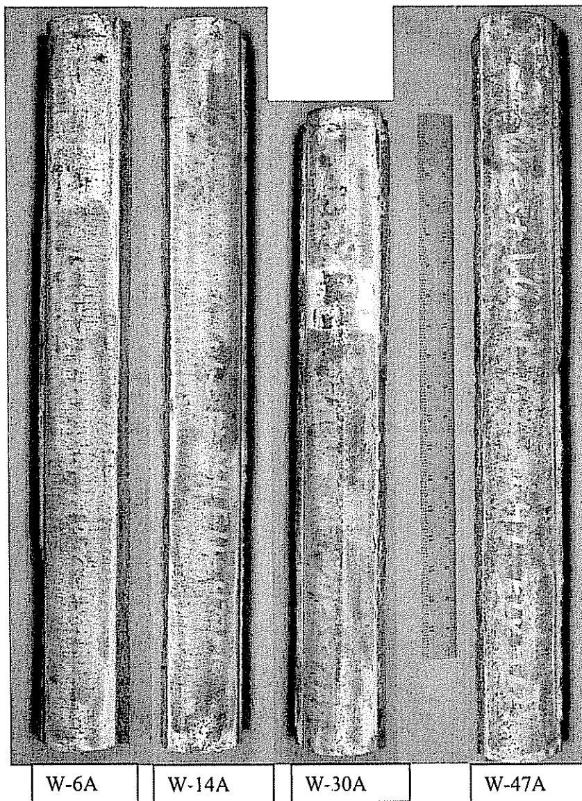
Figure 1. As-received tubes from the West Waterwall.
