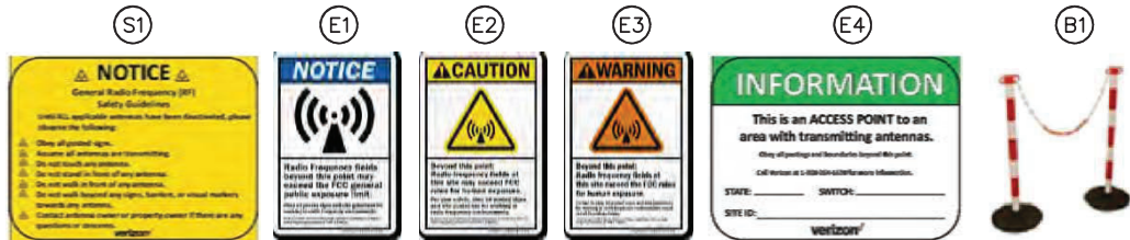
FIGURE 9 – TYPICAL E.M.E. SIGNAGE
