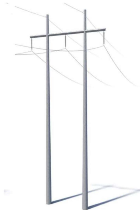
Figure 2. Typical Proposed Transmission Line Structure (Steel H-Frame) approximately 70 - 120 feet tall
