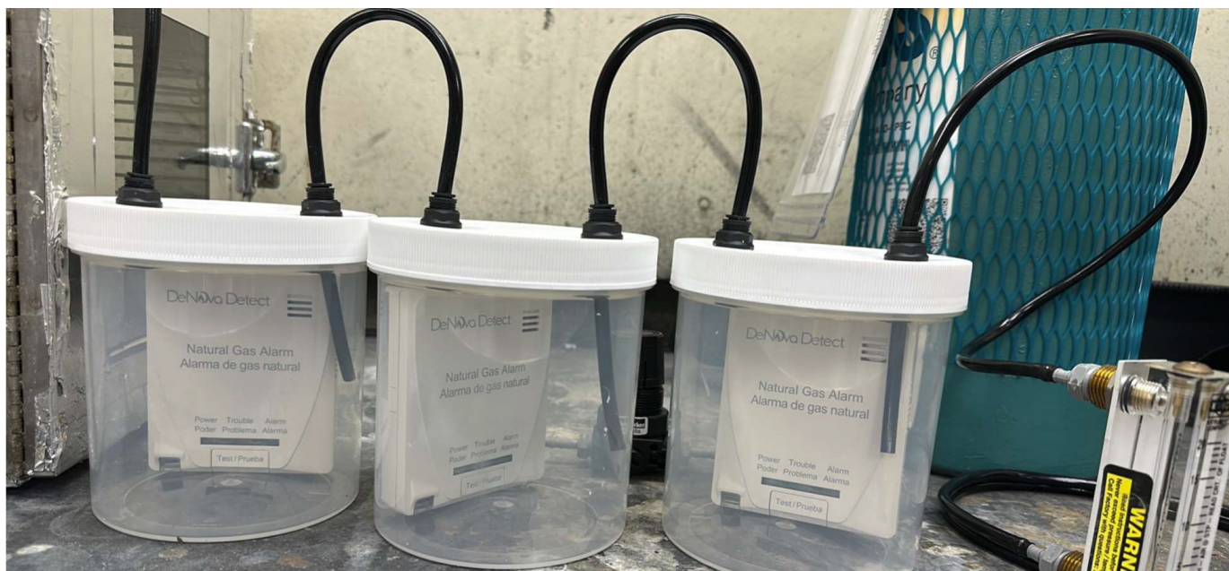
Simulation of below-ground leaks through soil during outdoor testing.
