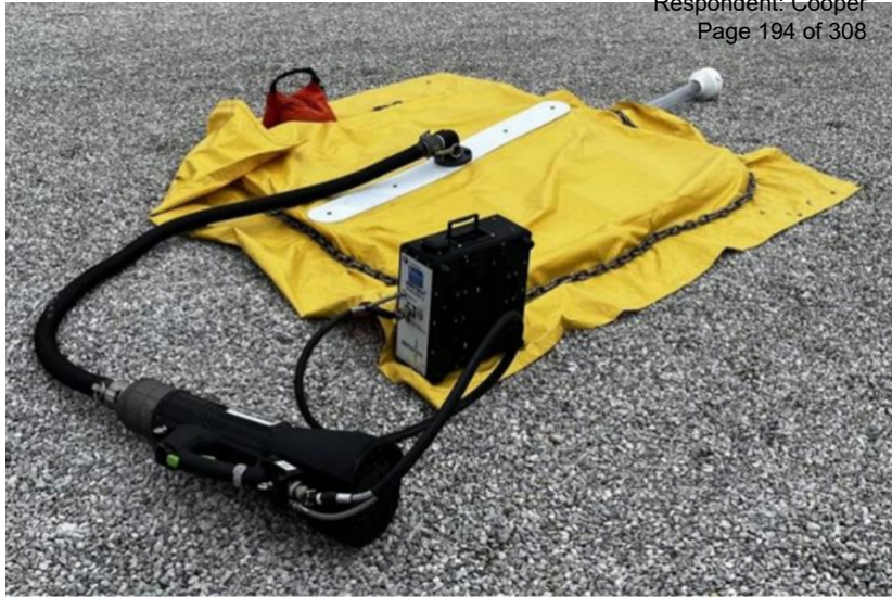
High flow sampler connected to tarp enclosure over a simulated leak
