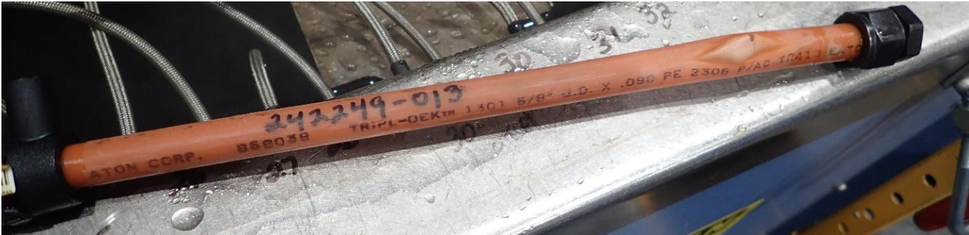
Specimen 242249-013, Ductile failure in pipe
