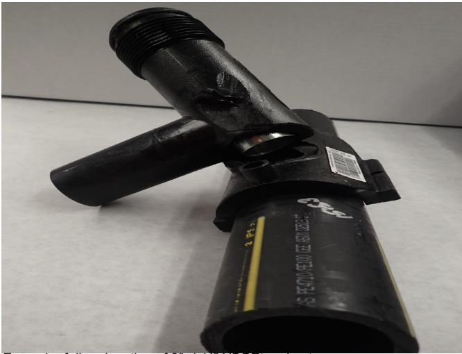
Exemplar failure location of 2"x1-1/4" HDPE tapping tee
