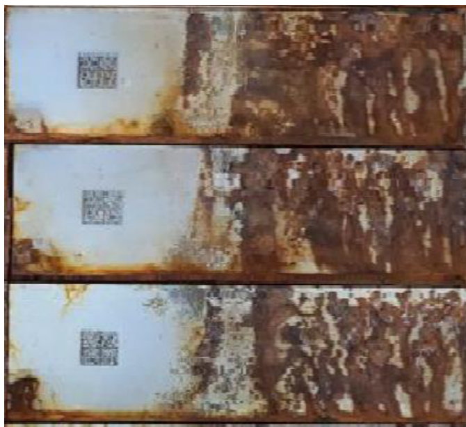
Fifty hours of salt spray. Untreated control barcode on right
