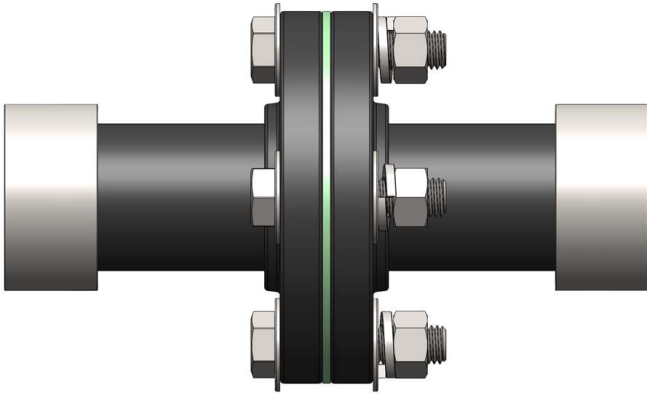
Proposed Black Steel 2 IPS Gasket Test Sample (Tapped 2 IPS Cap – 4in Long 2 IPS Pipe Nipple – Socket Weld 150 Class 2 IPS Pipe Flange – Test Gasket)
