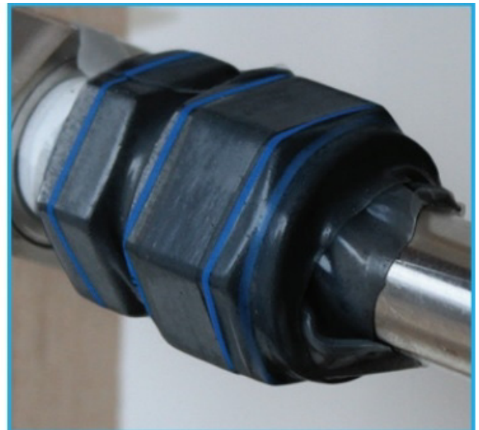
Hydrogen Leak Detected
