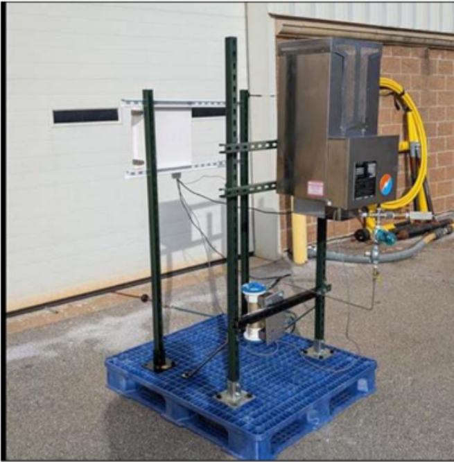
Test Stand for Thermoelectric Generator
