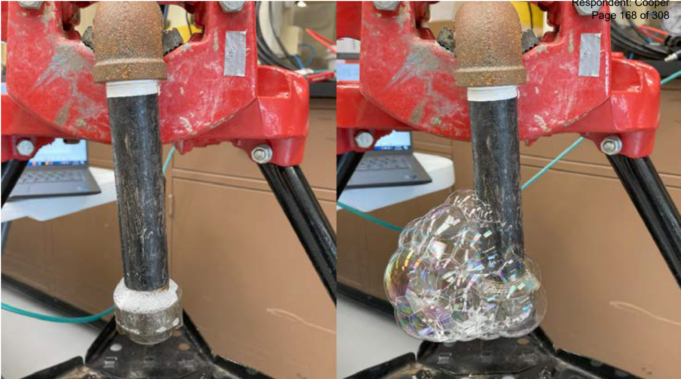
Two examples of laboratory testing and photos obtained. The left photo is a soap solution tested at 0.25 psi with a flow rate of 0.05 scfh. The right photo is a soap solution tested at 30 psi with a flow rate of 5 scfh.
