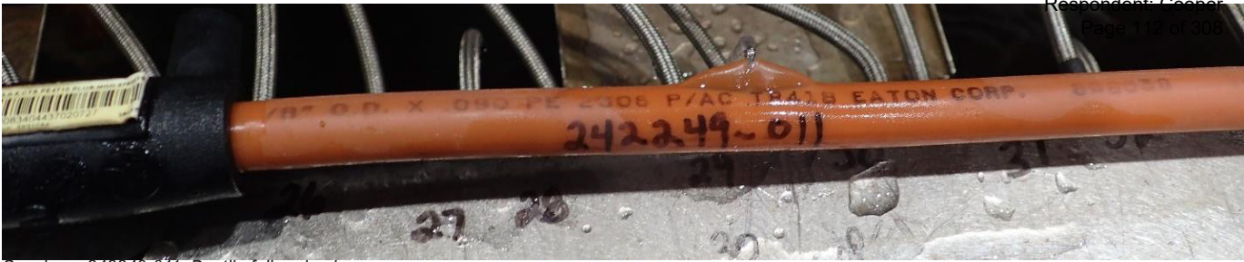
Specimen 242249-011, Ductile failure in pipe
