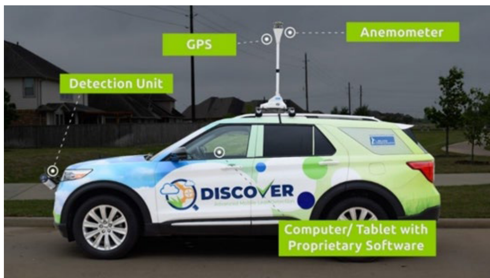
Discover AMLD system components (source: Discover Advanced Mobile Leak Detection- Product Brochure)
