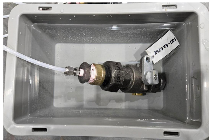
Gas Tightness Test setup
