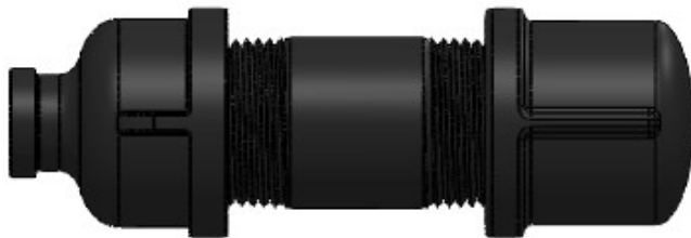
Black Steel 1 NPT Threaded Test Sample (1 NPT to 1/4 NPT Reducer – 3in Long 1 NPT Pipe Nipple – 1 NPT Cap)
