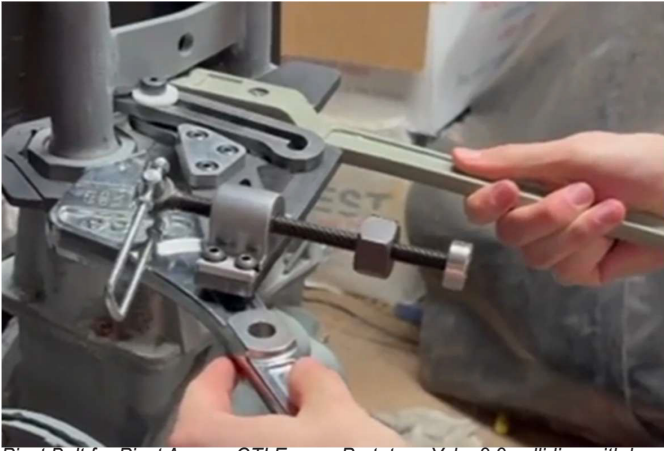
Pivot Bolt for Pivot Arm on GTI Energy Prototype Yoke 2.2 colliding with low clearance meter bar
