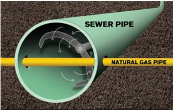
Plumbing Auger about to cut through Cross-Bore
