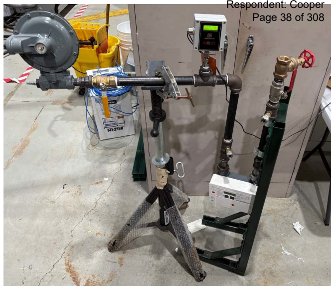
Meter Capacity Test Rig
