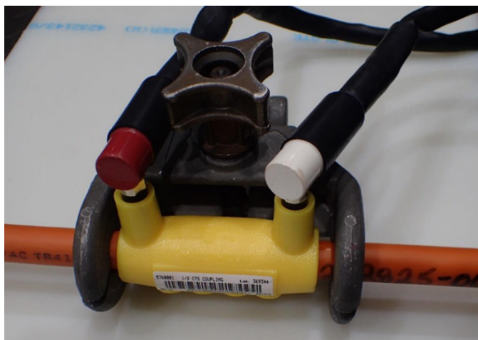
P/AC pipes being joined by a MDPE electrofusion coupling
