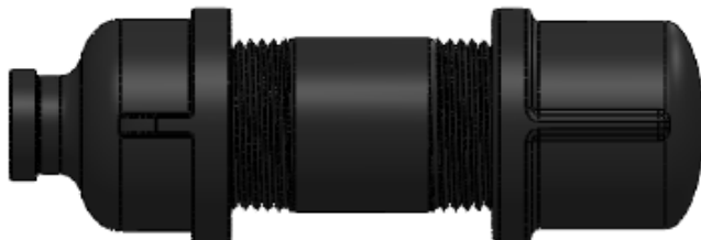
Black Steel 1 NPT Test Sample (1 NPT to 1/4 NPT Reducer – 3in Long 1 NPT Pipe Nipple – 1 NPT Cap)
