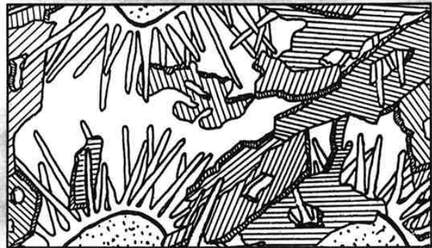
Hatched Areas: Crosslink structure of the epoxy resin lamina Ray Areas: Cement crystals formed before hydrating
