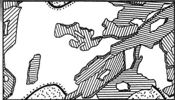
Hatched Areas: Crosslink structure of the epoxy resin lamina Dotted Areas: Cement grains before hydrating
