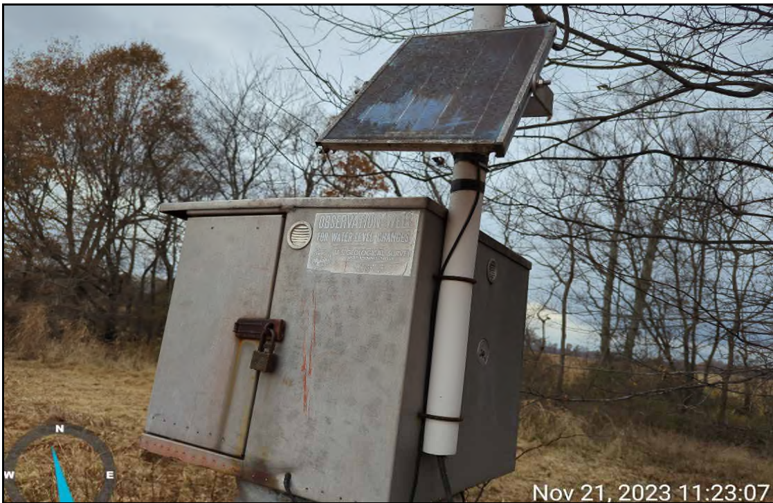
Photograph 28 – Parcel 57 – USGS monitoring well. November 21, 2023
