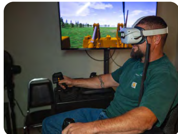
An EKPC employee uses a virtual reality training simulator to hone their skills on working the coal pile.
