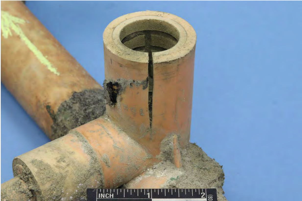
Figure 13. Longitudinal fracture in retired service tee.
