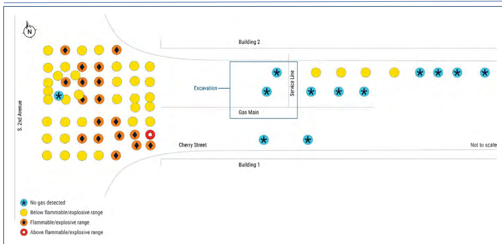
Figure 9. Bar hole test readings conducted in March 2023 ( left side of image ) and April 2023 ( right side of image ).
