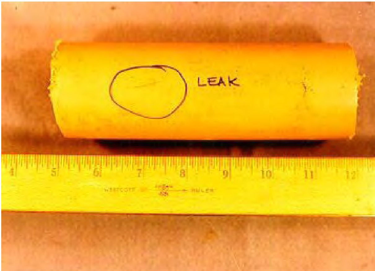
Figure 6 -- Slit fracture on a polyethylene pipe manufactured by DuPont that was found leaking and removed from a gas piping system.
