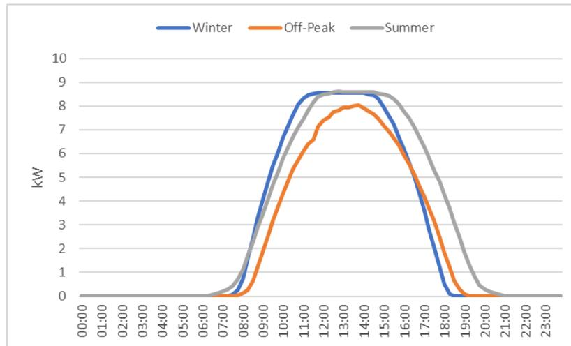
Figure 2 - Solar production profiles used during the analysis. All data was captured from the LG&E and KU Simpsonville Solar Share facility.<sup>2</sup> Note that only the 10 kW array size profiles are shown here and a 1.2 DC to AC ratio was assumed.
