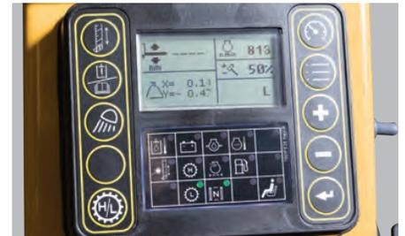
**AT YOUR FINGERTIPS.** An industry-unique integrated control system offers the operator a variety of machine information, including pile angle and height. Display also shows machine maintenance information to help maintain service schedules.
