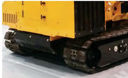
**LEAVE IT LIKE YOU FOUND IT.** The PD10 features a wide track pad to minimize jobsite disturbance in widely varying ground conditions.
