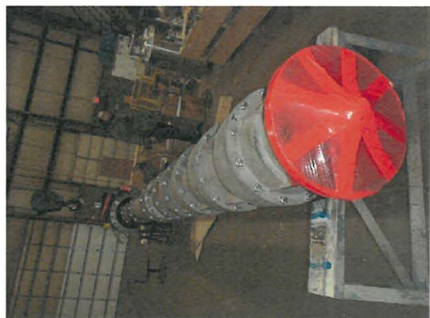
Photo 2: Completed Pump Assembly
