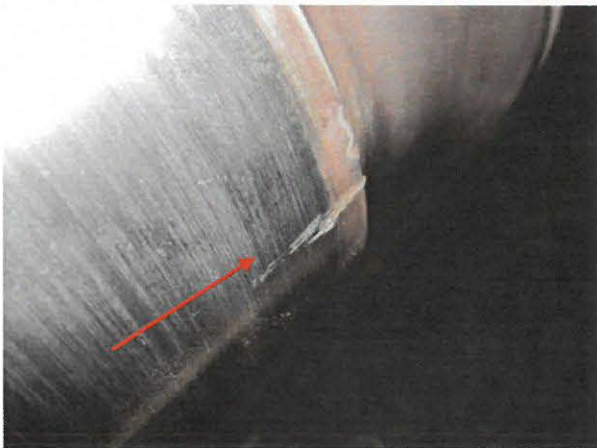
Photo 3: Shaft Gall At Balance Sleeve Fit
