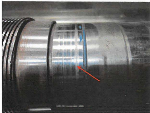
Photo 4: Shaft Wear From Bearing Covers
