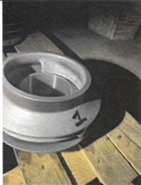
Linears found on vane inlets and outlets
