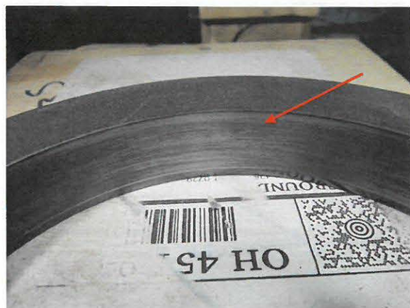
Photo 12: Typical Wear On Stage Pieces
