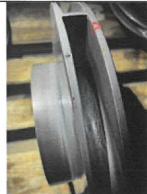
Linear found on vane outlet.
