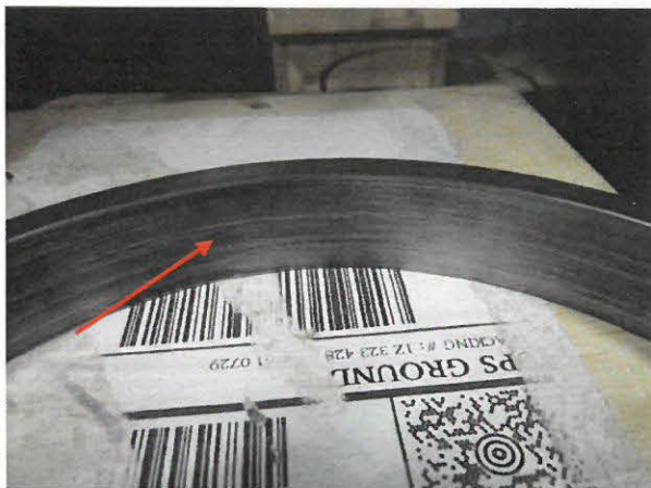
Photo 11: Typical Wear On Case Rings
