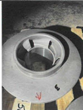
Linears found on vanes and keyway.
