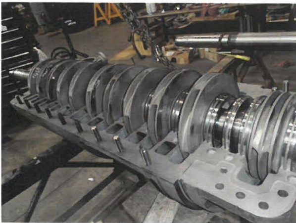
Photo 3: Rotor Cradle Check In Casing
