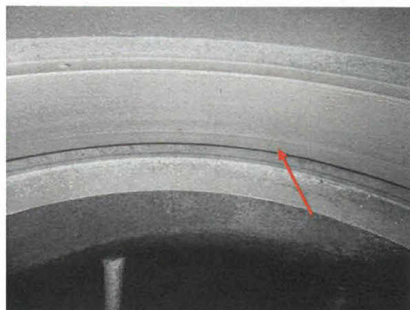
Photo 4: Typical Case Ring Wear
