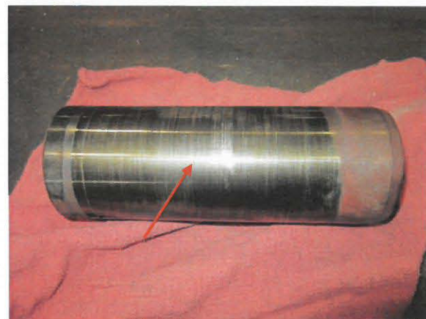
Photo 10: Wear On Suction Shaft Sleeve
