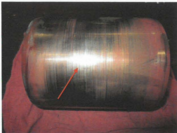
Photo 9: Typical Wear On Series Shaft Sleeves
