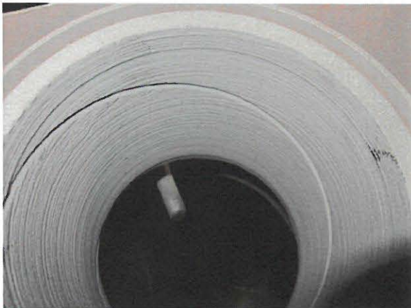
Photo 7: Typical Wear On Series Bearing
