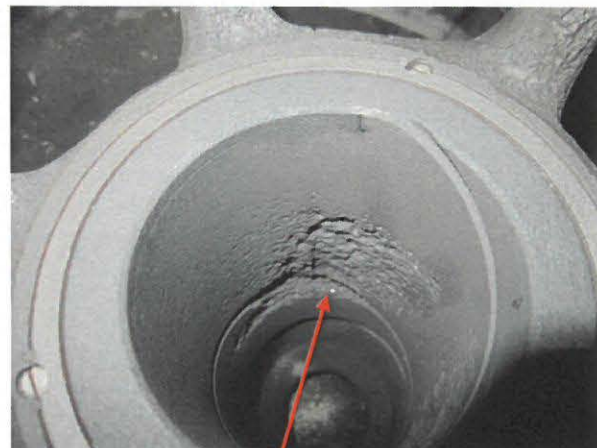
Photo 8: Cavitation Damage On Suction Bearing
