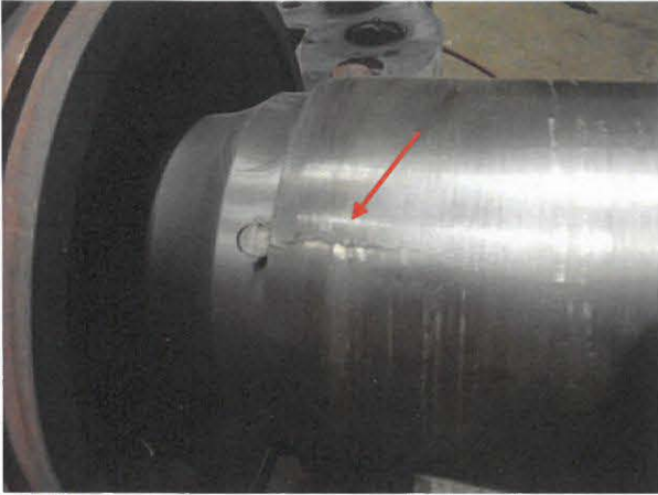
Photo 5: Cracked Balance Sleeve (As Received)
