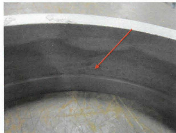
Photo 10: Fretting In Volute Bushing Bore
