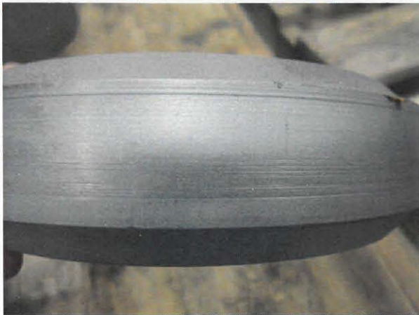
Photo 7: Light Wear On 1-2 Sleeve Turn
