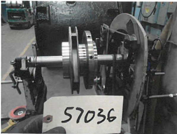
Photo 1: Center Impeller Assembly Balance
