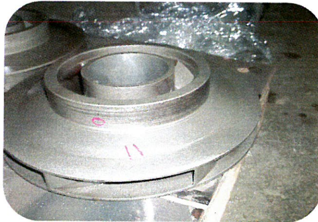
Linear indications found on hub turn from 1/16" – 3/16".
