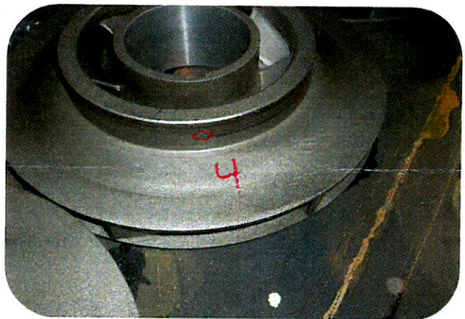
Linear indications found on hub turn from 1/16" – 3/16".
