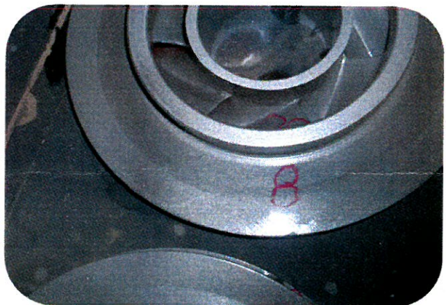
Linear indications found on hub turn and vane inlet from 1/16" - 1/4".
