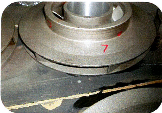
Linear indications found on hub turn from 1/16" - 1/8".
