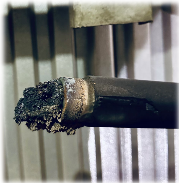
Figure 6: Melted HVT Probe Tip
