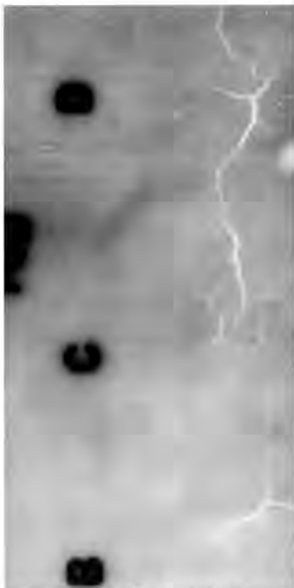
6. Radiographic films illustrate surface fissuring on the inside arc of a pipe bend
