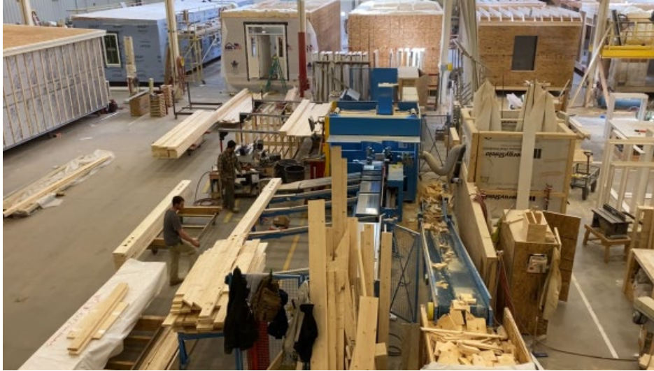
Figure A18. Mill Room/Automated Computer Driven CNC Saw.
