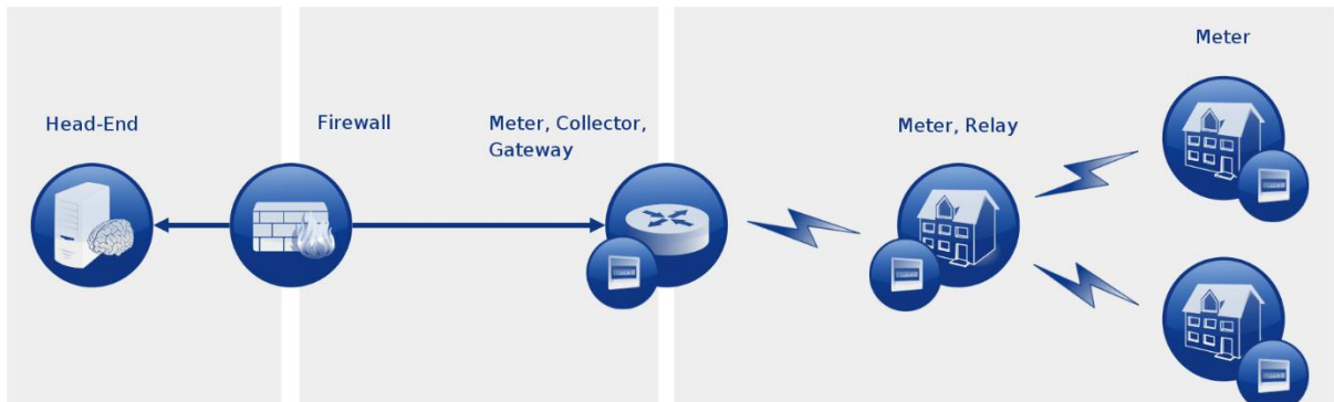
Figure SDB-1: AMI Communication System Interface
