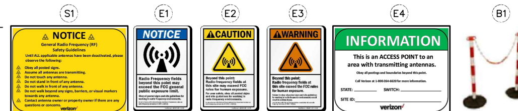
FIGURE 9 - TYPICAL E.M.E. SIGNAGE
