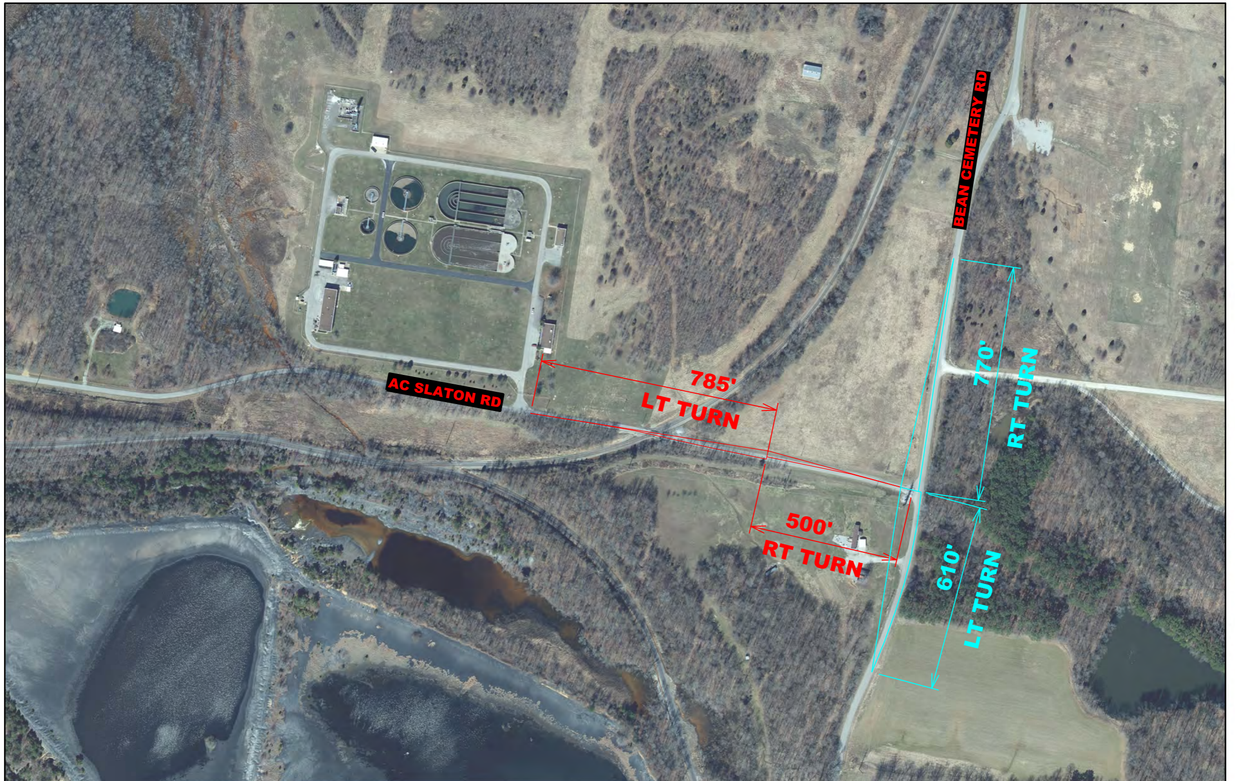
FIGURE 4 SIGHT DISTANCE TRIANGLES
