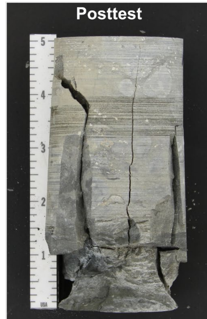
Figure D-10. Unconfined Compression and Constant Strain Rate Test Plots and Pre- and Posttest Photographs of Specimen NFRONT/MAD-21/127.4.
