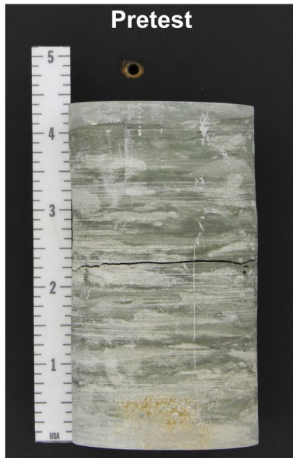
Figure D-2. Unconfined Compression and Constant Strain Rate Test Plot and Pre- and Posttest Photographs of Specimen NFRONT/MAD-05/99.6.
