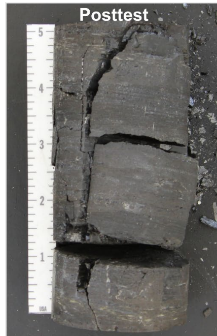
Figure D-4. Unconfined Compression and Constant Strain Rate Test Plots and Pre- and Posttest Photographs of Specimen NFRONT/MAD-09/134.8.
