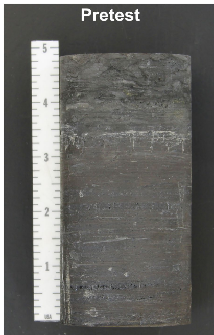
Figure D-8. Unconfined Compression and Constant Strain Rate Test Plots and Pre- and Posttest Photographs of Specimen NFRONT/MAD-16/122.4.
