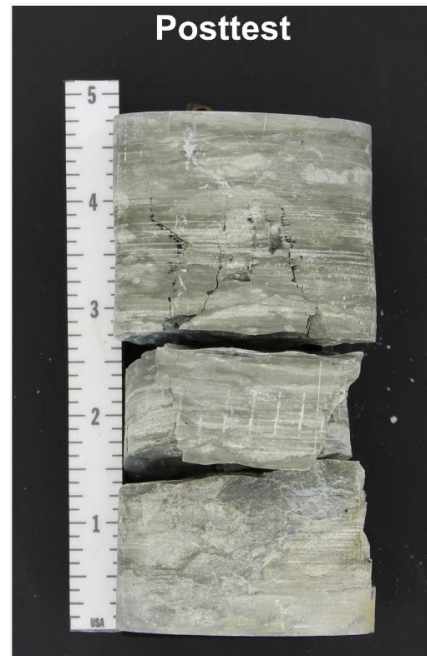
Figure D-2. Unconfined Compression and Constant Strain Rate Test Plot and Pre- and Posttest Photographs of Specimen NFRONT/MAD-05/99.6.
