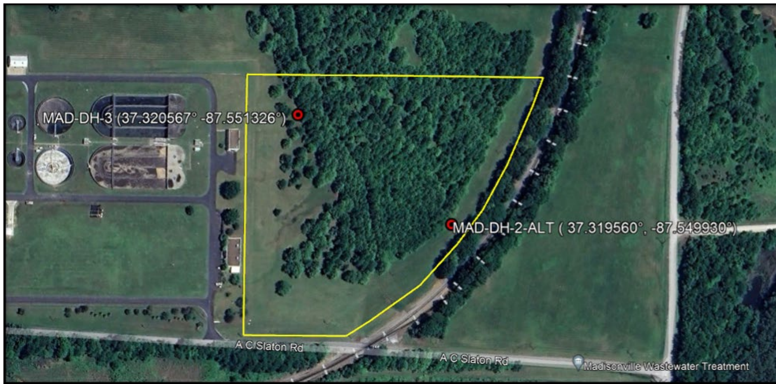
Figure B-26. Approximate Locations of the Two Drillholes Drilled on the Madisonville Property.
