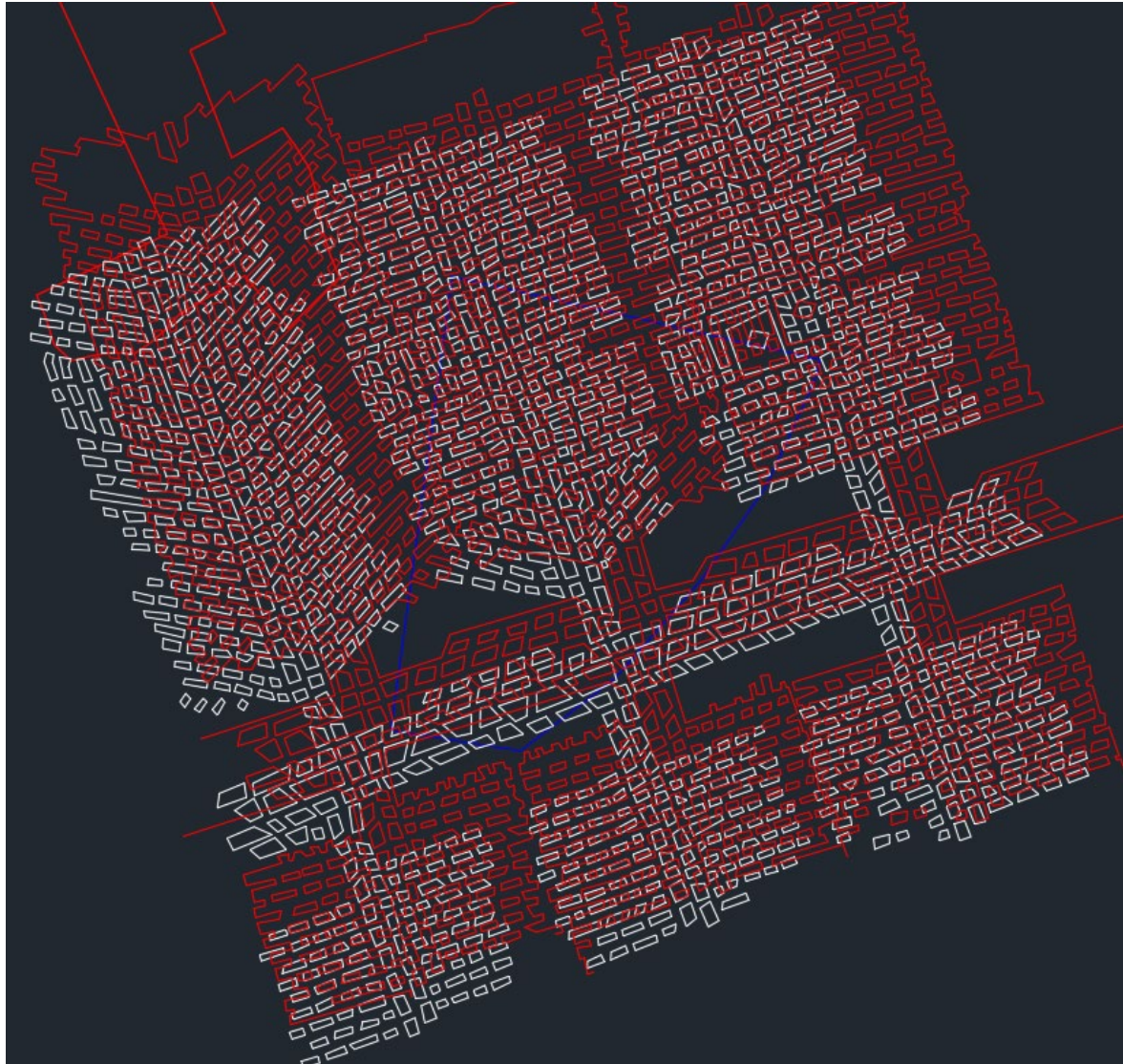
Figure B-2. Comparison of the Kentucky Geological Survey (White) and RESPEC Georeferenced (Red) Mine Maps for WKY 11.
