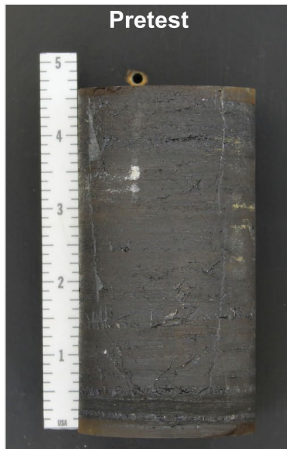
Figure D-5. Unconfined Compression and Constant Strain Rate Plots and Pre- and Posttest Photographs of Specimen NFRONT/MAD-10/137.1.
