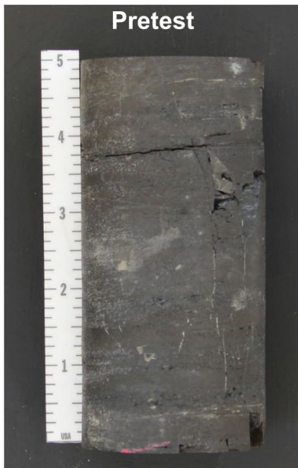
Figure D-4. Unconfined Compression and Constant Strain Rate Test Plots and Pre- and Posttest Photographs of Specimen NFRONT/MAD-09/134.8.
