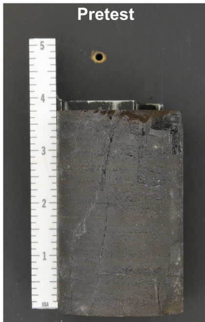
Figure D-6. Unconfined Compression and Constant Strain Rate Test Plots and Pre- and Posttest Photographs of Specimen NFRONT/MAD-10/143.0.
