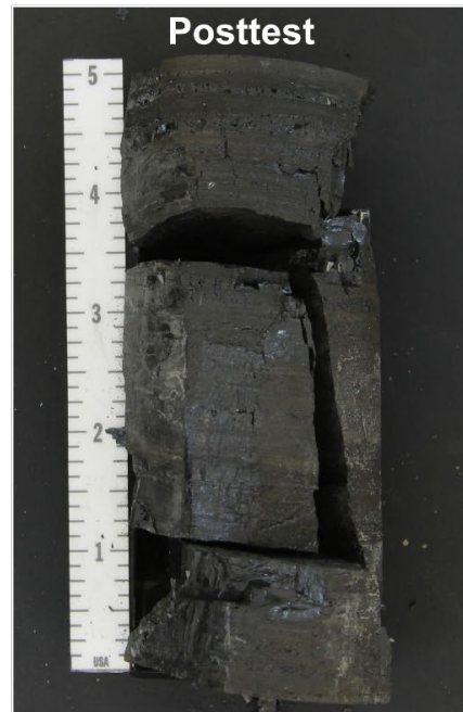
Figure D-5. Unconfined Compression and Constant Strain Rate Plots and Pre- and Posttest Photographs of Specimen NFRONT/MAD-10/137.1.
