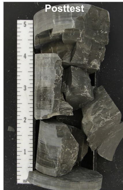
Figure D-15. Unconfined Compression and Constant Strain Rate Test Plots and Pre- and Posttest Photographs of Specimen NFRONT/MAD-28/228.5.
