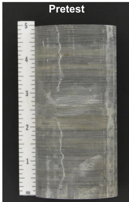
Figure D-15. Unconfined Compression and Constant Strain Rate Test Plots and Pre- and Posttest Photographs of Specimen NFRONT/MAD-28/228.5.
