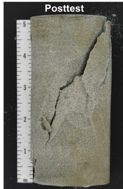
Figure D-14. Unconfined Compression and Constant Strain Rate Test Plots and Pre- and Posttest Photographs of Specimen NFRONT/MAD-24/206.2.
