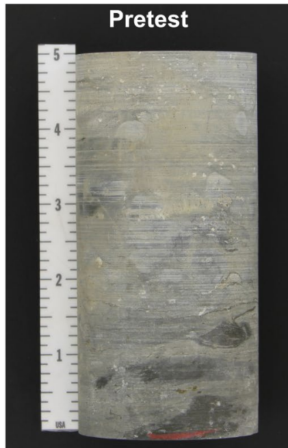
Figure D-10. Unconfined Compression and Constant Strain Rate Test Plots and Pre- and Posttest Photographs of Specimen NFRONT/MAD-21/127.4.
