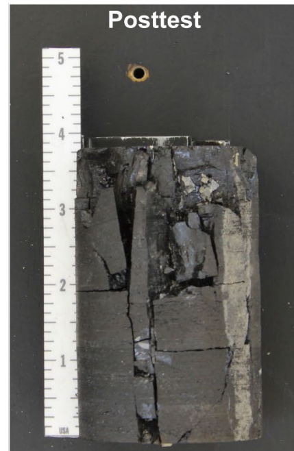
Figure D-6. Unconfined Compression and Constant Strain Rate Test Plots and Pre- and Posttest Photographs of Specimen NFRONT/MAD-10/143.0.
