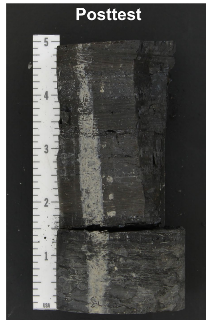
Figure D-8. Unconfined Compression and Constant Strain Rate Test Plots and Pre- and Posttest Photographs of Specimen NFRONT/MAD-16/122.4.
