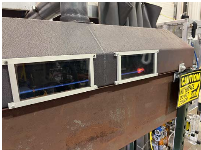
Ribbon burner test setup in laboratory
