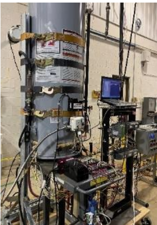
Water heater with damper, data acquisition system and water load simulator for testing (left). Programmable water load simulator (right)
