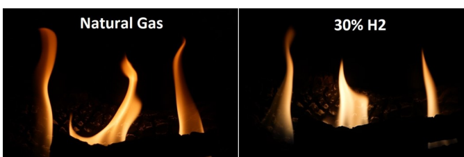
Hearth testing with Natural Gas (left) and a 30% H2 blend (right)
