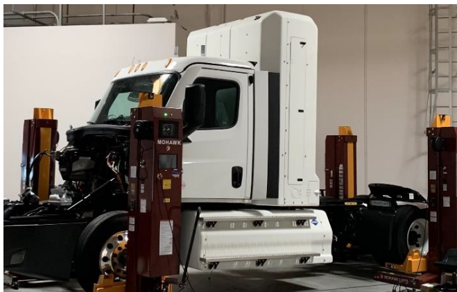
Hydrogen tanks installed on the truck
