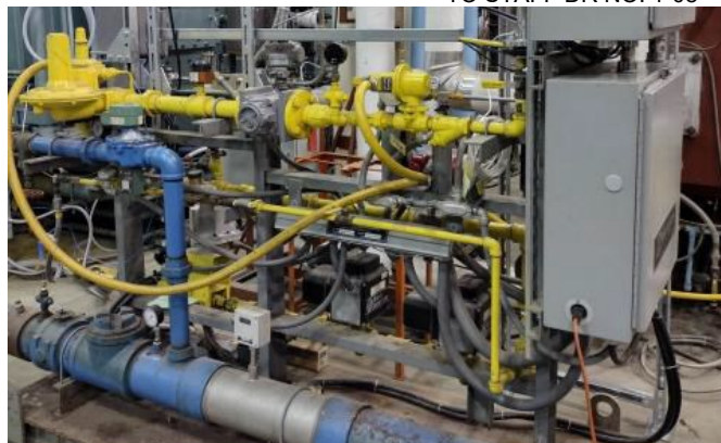
Air-fuel skid assembly for H2 operation
