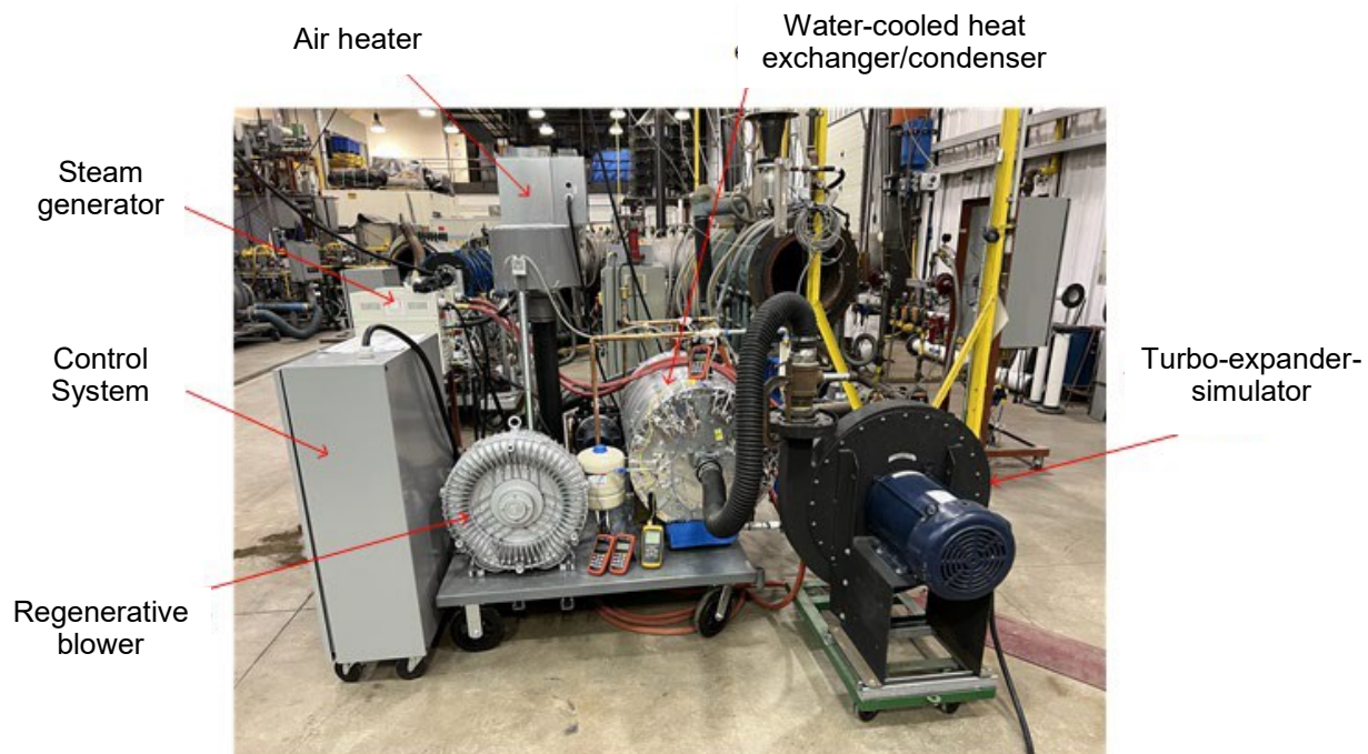
Overall view of the PDHS prototype installed and tested in the laboratory.
