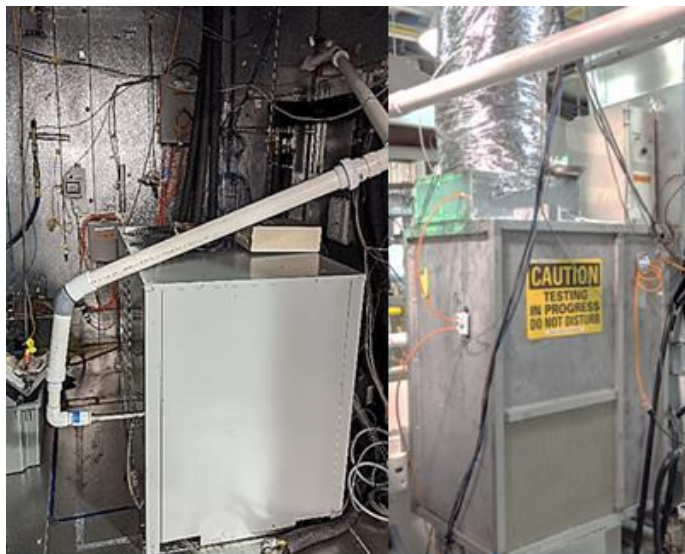
SMTI 40K Hybrid GAHP system installation in HVAC laboratory. (left) The installation of the GAHP in a environmental chamber; (right)
