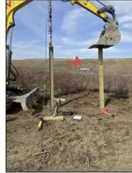
Figure 2: Typical Uplift Test Setup
