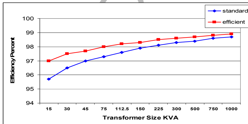
Figure 31. Transformer Efficiency Specification NEMA TP-1
