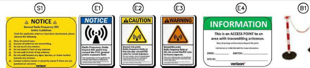
FIGURE 9 - TYPICAL E.M.E. SIGNAGE
