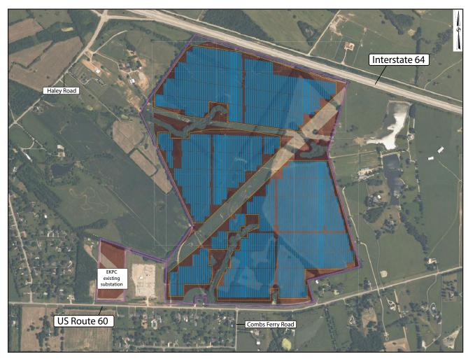
Cooperative Solar Farm Two - Fayette will feature photovoltaic (PV) solar panels mounted on single-axis tracking systems supported by steel posts. When operating, the solar panels will move to track the sun from east to west over the course of the day. The solar farm will have capacity to generate 40 megawatts of electricity at alternating current (AC). That is enough to serve the annual electricity needs of 4,560 typical Kentucky homes.
