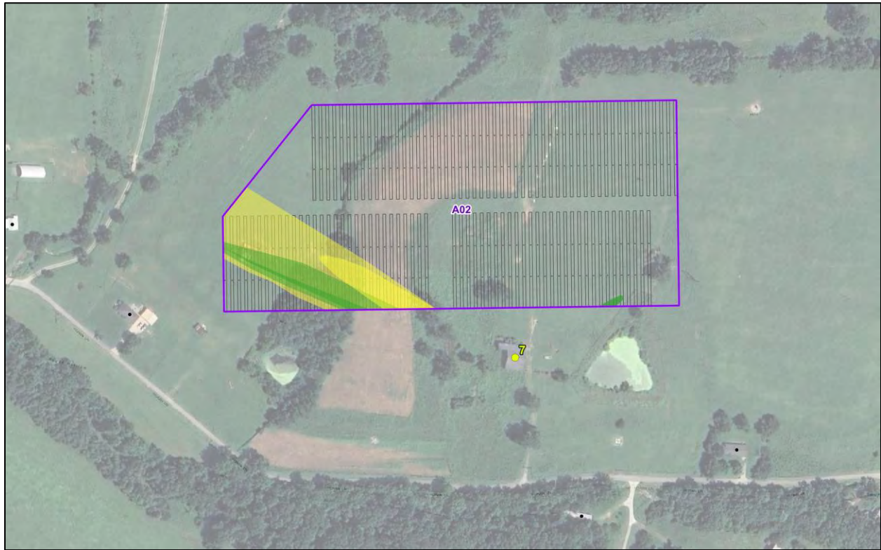
Figure 7: Discrete observation point 7 (yellow point) receiving glare from Sub-Array A02
