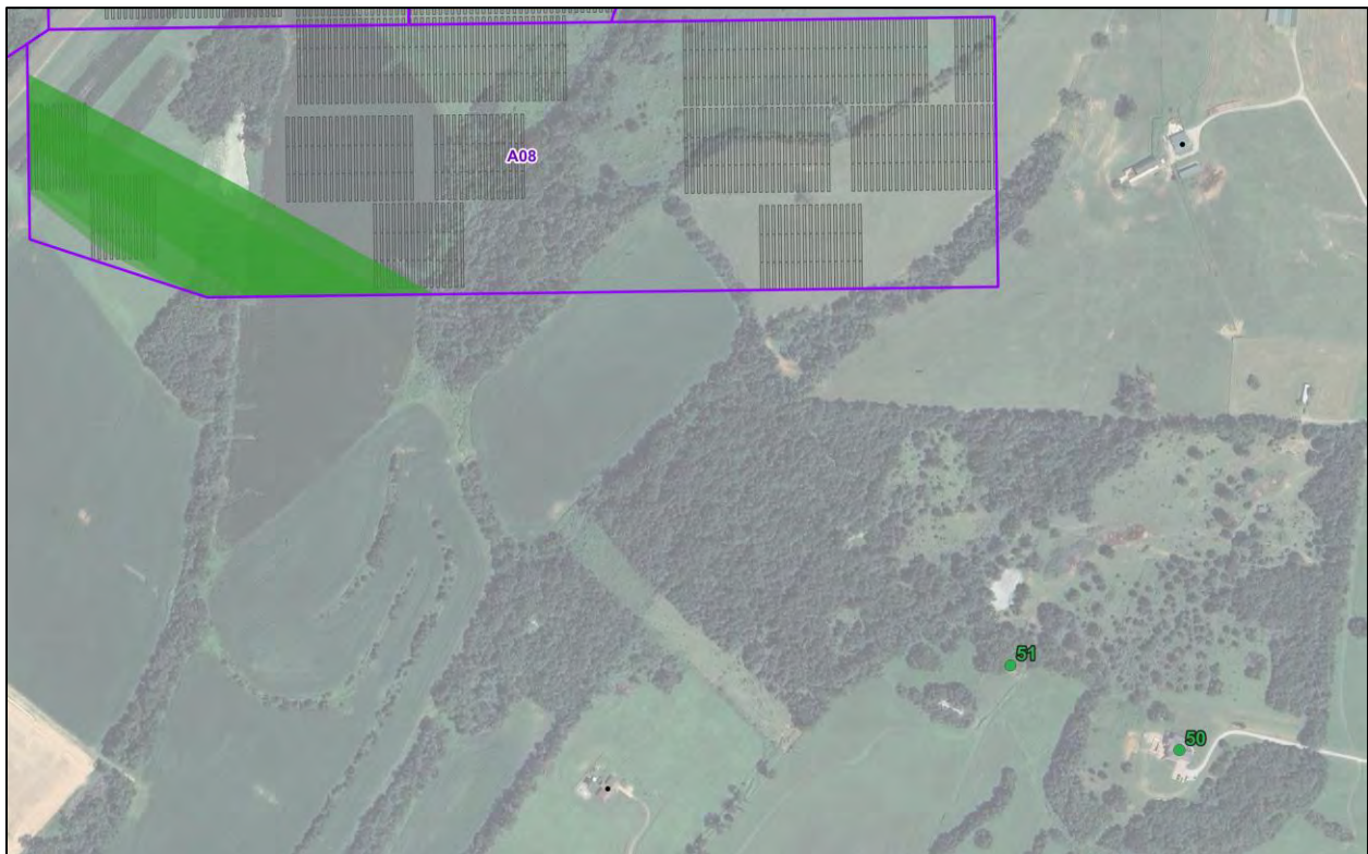
Figure 9: Discrete observation points 50 and 51 (green points) receiving glare from Sub-Array A08
