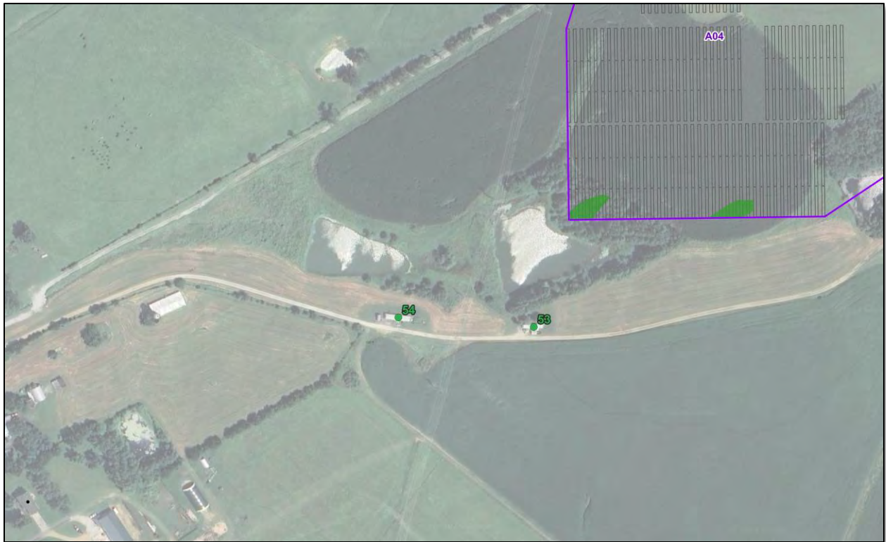
Figure 10: Discrete observation points 53 and 54 (green points) receiving glare from Sub-Array A04
