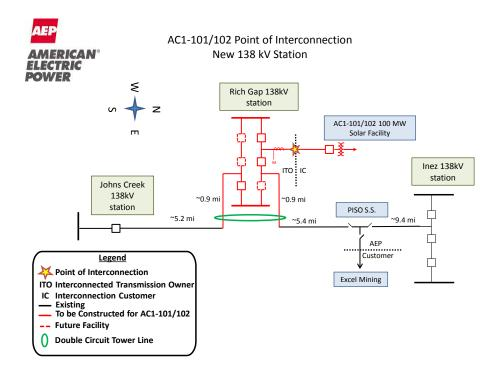
The Point of Interconnection is the first structure outside of the new 138 kV station (such structure being located in Interconnection Customer's Collector Substation) with the Interconnected Transmission Owner owning the first span of conductors, and the Interconnection Customer owning the first structure.
