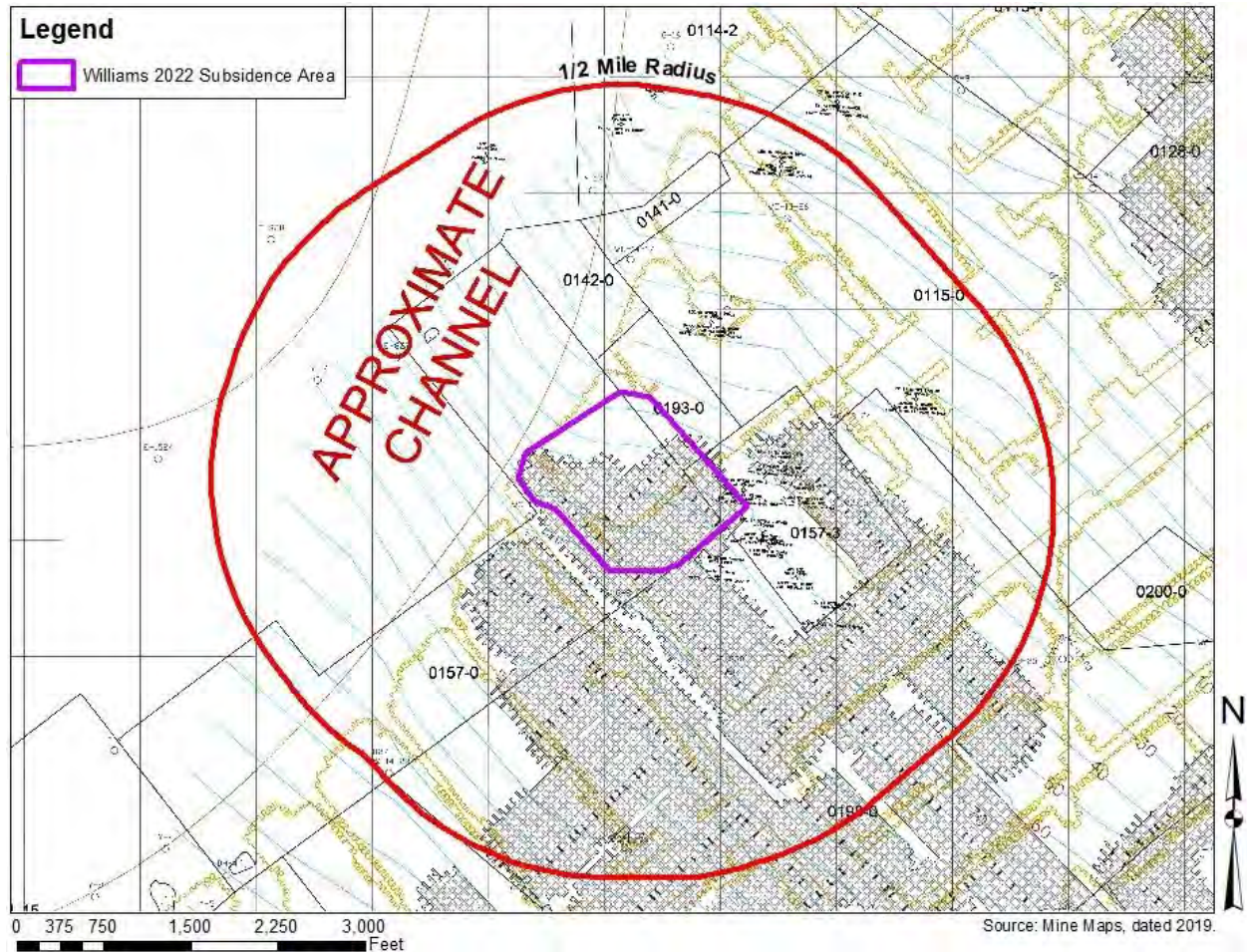
Figure 4. 2019 Mine Maps showing documented coal mining in the No. 13 seam within ½ mile radius of the Williams property, by Webster County Coal LLC, Permit Nos. 917-5023 and 917-5013.
