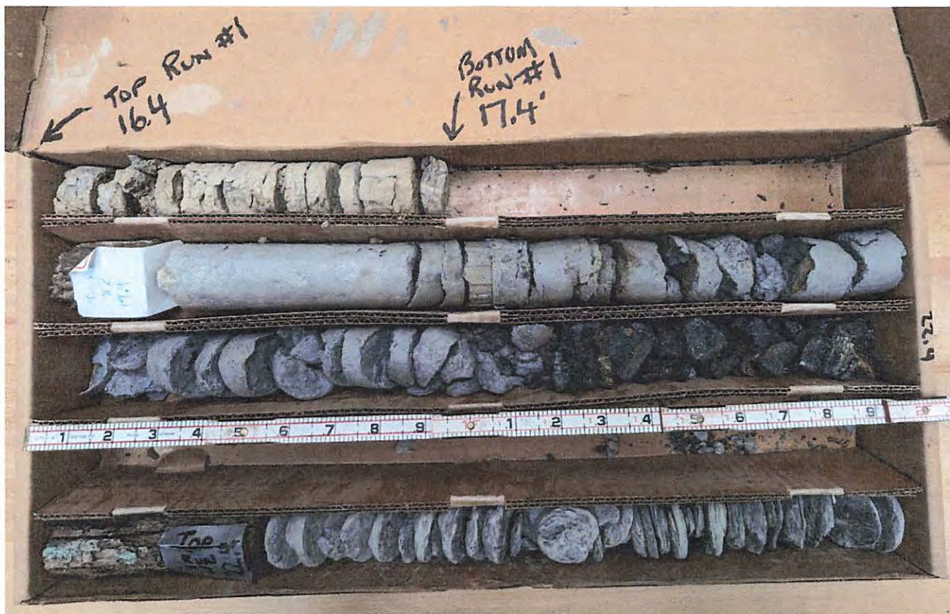
Rock Core Photo: 16.4 feet to 24.4 feet below ground surface.
