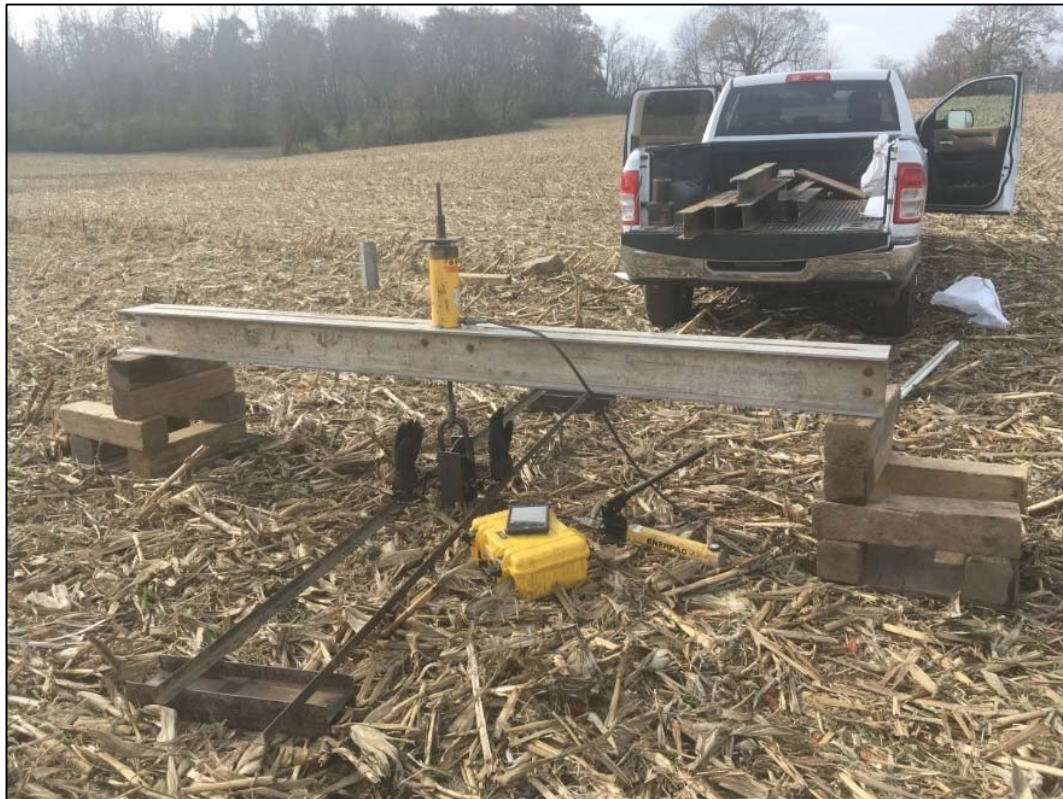
Post Tension Load Test Setup
