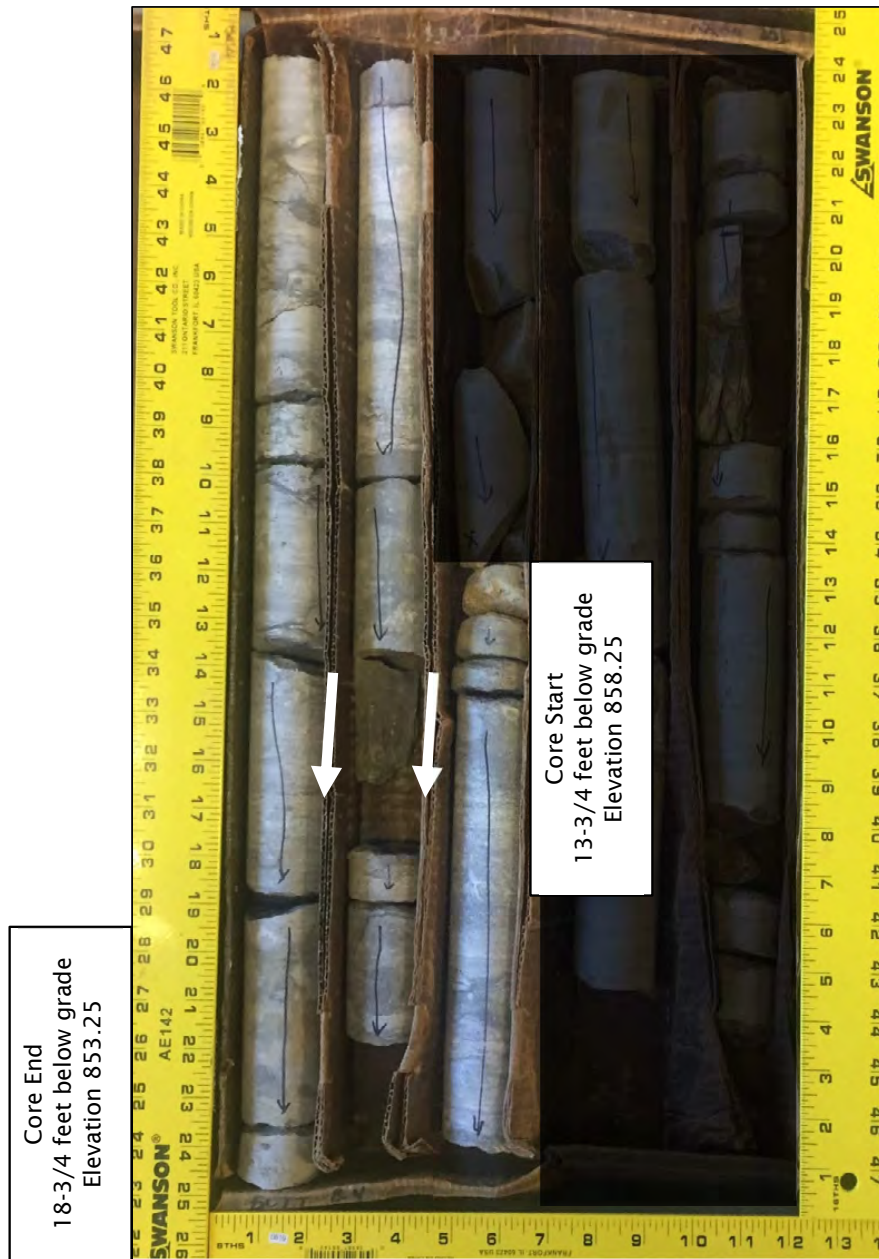
Rock Core B-4 RC-5 (5 Feet) 13-3/4 feet to 18-3/4 feet below grade (El. 858.25 to El. 853.25) Moderately Strong Gray Faintly Weathered Limestone Recovery: 93% RQD: 60% Coring Rate: 0.08 to 0.10 in/sec
