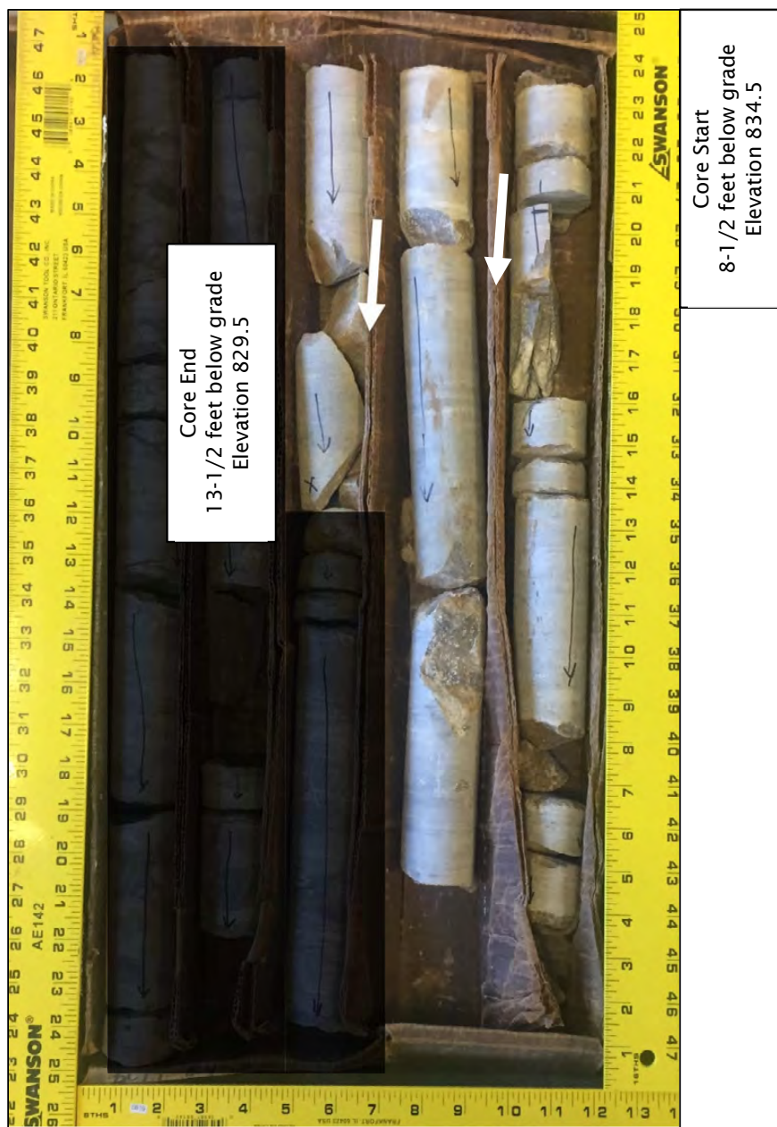
Rock Core B-12 RC-4 (5 Feet) 8-1/2 feet to 13-1/2 feet below grade (El. 834.5 to El. 829.5) Moderately Strong Gray Faintly Weathered Limestone Recovery: 82% RQD: 58% Coring Rate: 0.09 to 0.11 in/sec
