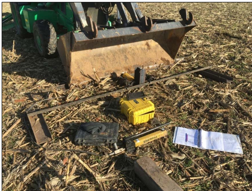
Post Lateral Load Test Setup
