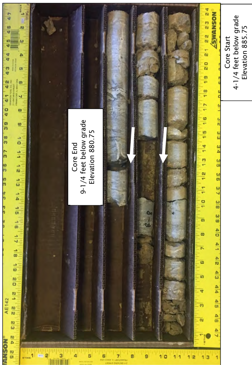
Rock Core B-8 RC-3 (5 Feet) 4-1/4 feet to 9-1/4 feet below grade (El. 885.75 to El. 880.75) Moderately Strong Gray Faintly Weathered Limestone Recovery: 88% RQD: 30% Coring Rate: 0.08 to 0.10 in/sec
