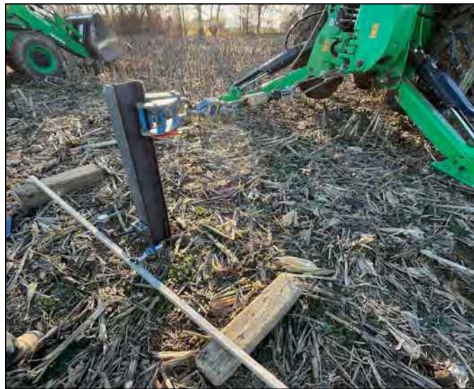
Lateral Load Test Setup
