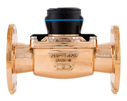
The MACH 10® ultrasonic water meter features solid state ultrasonic technology including a factory-calibrated, replaceable unitized measuring element (UME) with no degradation of accuracy over time. Combined with a corrosion-resistant, lead free, high-copper alloy maincase, the MACH 10 is built to withstand demanding service conditions and deliver sustained accuracy over the life of the meter.
