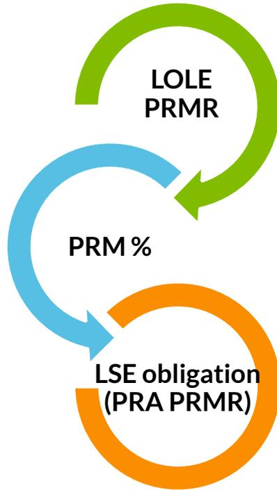
MISO determines the PRMR through completion of the seasonal Loss of Load Expectation (LOLE) study. The PRMR is equal to the total capacity needed to meet a LOLE of 1 day in ten years.
