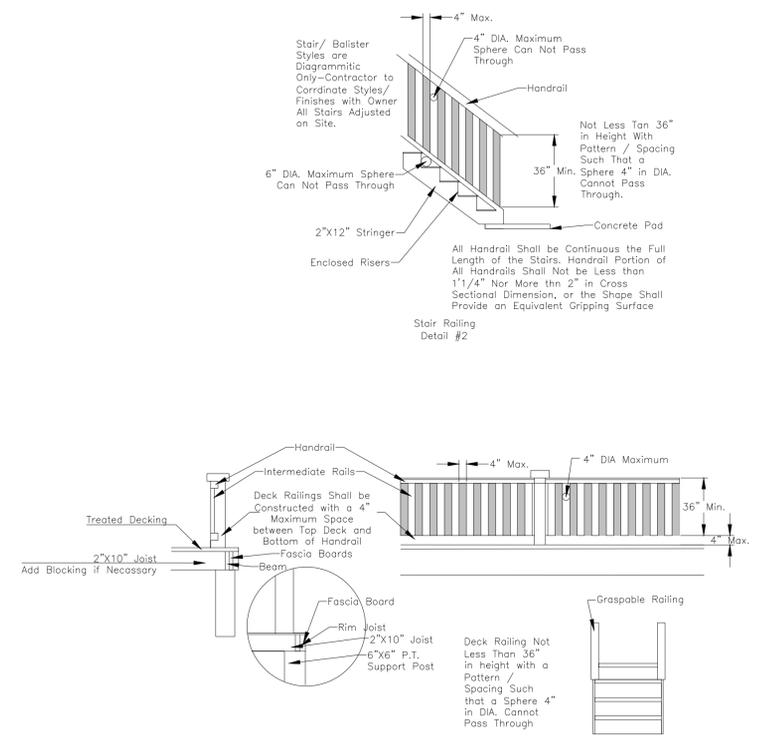
**WOOD DECK AND STAIR DETAIL (TVL-681,682 AND P-621 ACCESS PLATFORM)**
