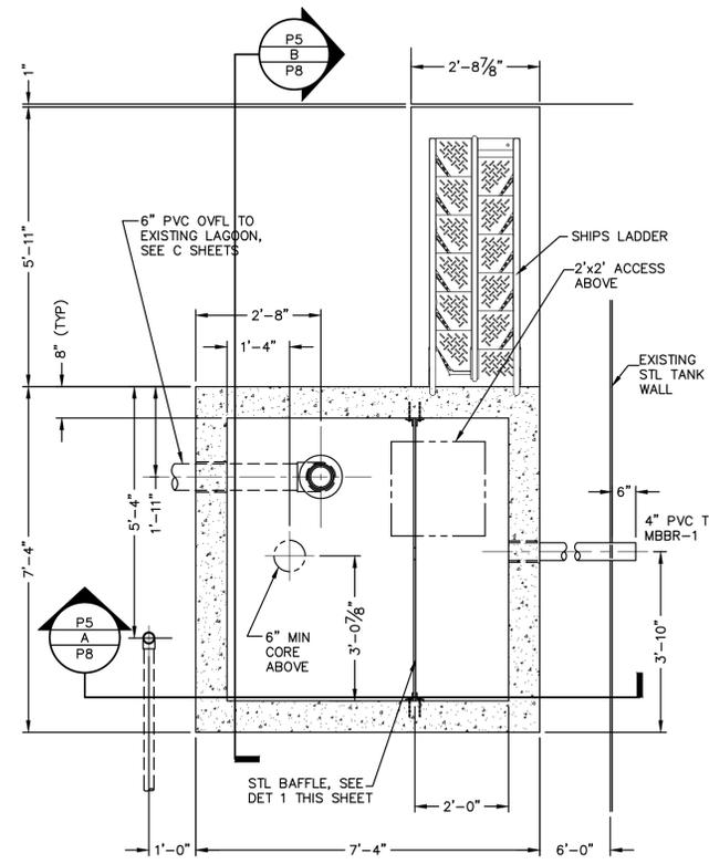
OVERFLOW STRUCTURE LOWER PLAN
