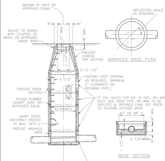
**PRE-CAST CONCRETE MANHOLE FOR SEWERS 8\"/>**
