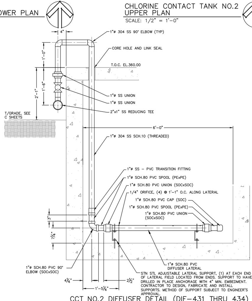
CCT NO.2 DIFFUSER DETAIL (DIF-431 THRU 434)
