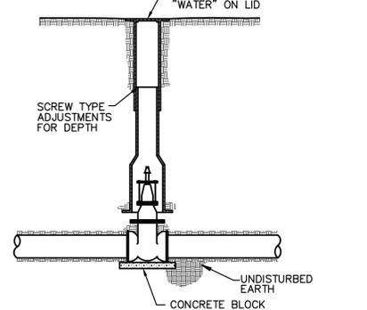
**TYPICAL VALVE BOX INSTALLATION**
