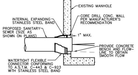
**PIPE TO MANHOLE CONNECTION**
