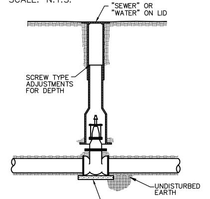
TYPICAL VALVE BOX INSTALLATION SCALE: N.T.S.
